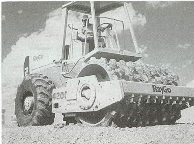
FIGURE 4 Roller for size reduction.
