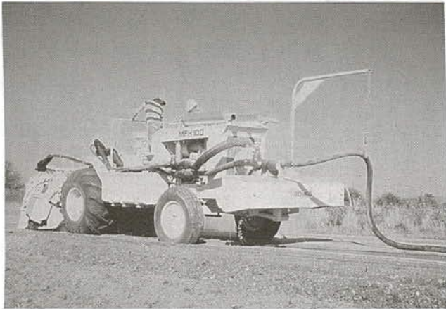
FIGURE 9 Transverse-shaft mixer for mixing.
