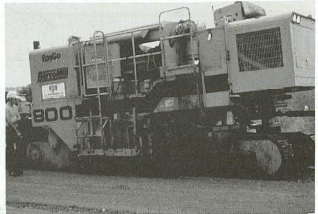
FIGURE 15 Cold-milling machine (RayGo).
