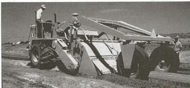
FIGURE 24 Single transverse-shaft rotary mixer.
