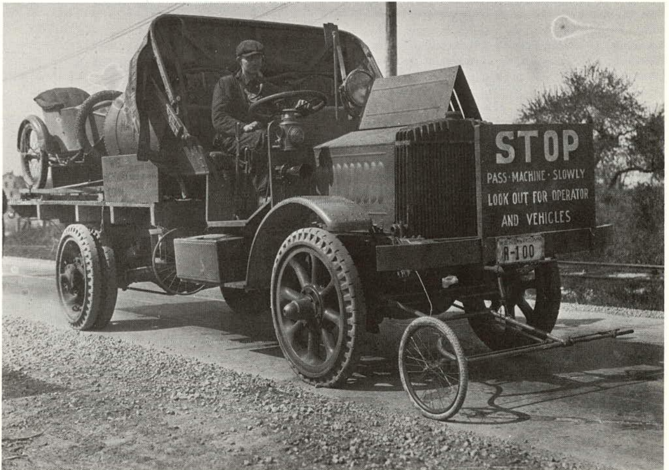
Figure 2. Early motor-driven striper. (Wisconsin Dept. of Trans.).
