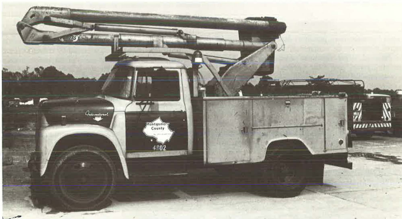
Figure 6. Cherry picker for signal maintenance.
