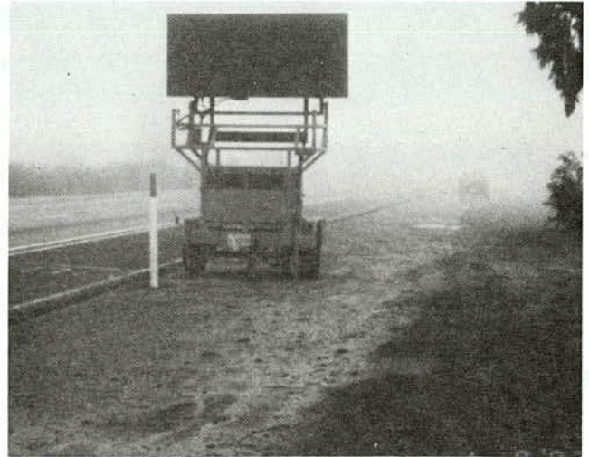
FIGURE 2 Portable changeable message sign in fog location.
