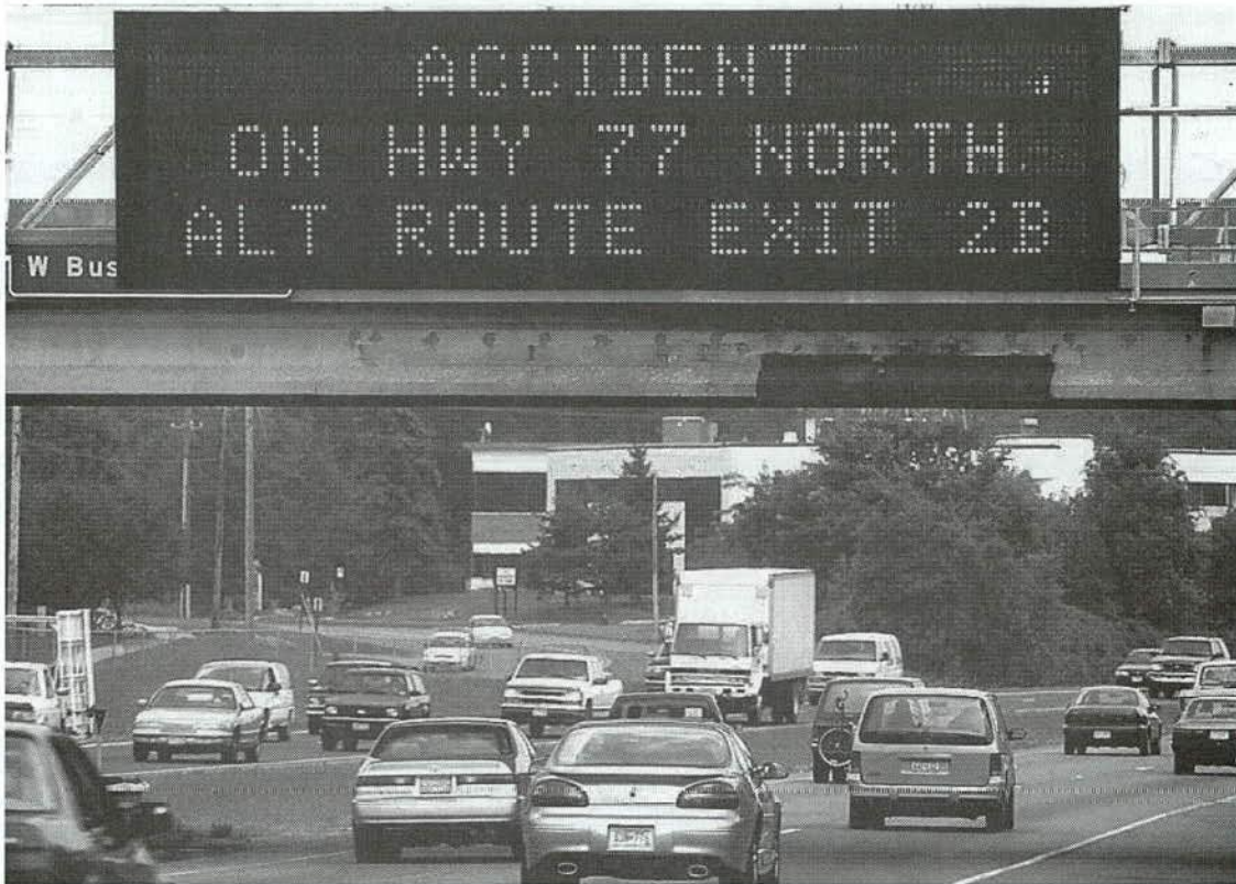
FIGURE 9 Among the most commonly used means for providing alternate route information are changeable message signs located upstream of the alternate route access point. (Photo courtesy of the Minnesota DOT.)
