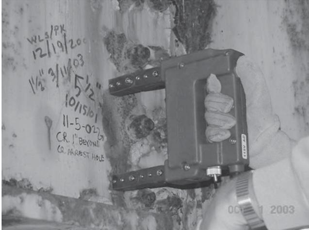
FIGURE A6 Magnetic particle testing—Placement of magnetic field.
