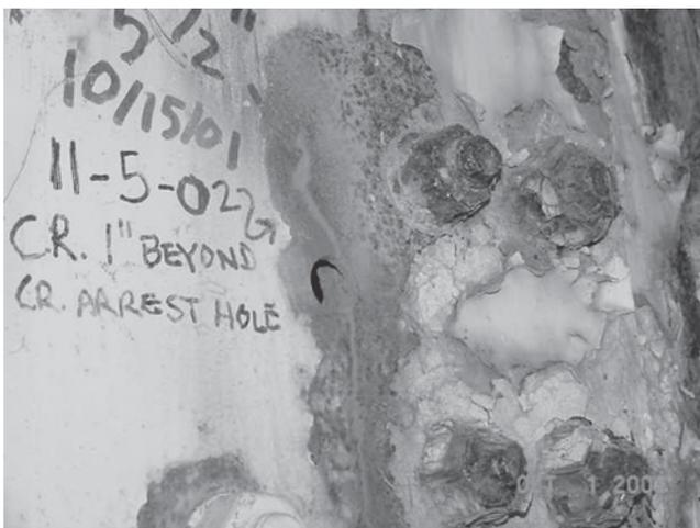
FIGURE A8 Magnetic particle testing—Indication.
