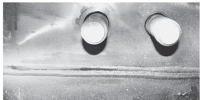
FIGURE A5 Example of indication from dye penetrant inspection.
