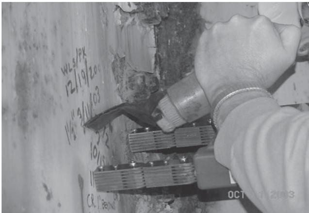
FIGURE A7 Magnetic particle testing—Application of magnetic particles.
