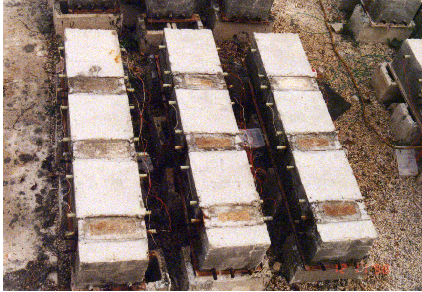
Figure C-4: Photograph of three G-109 macrobeams subsequent to fabrication and demolding.
