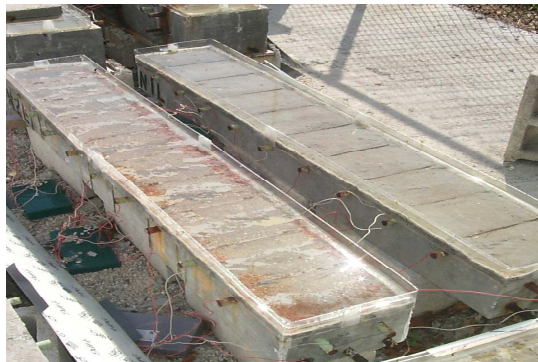
Figure B-11: Photograph of two NCD macrobeams under exposure testing.
