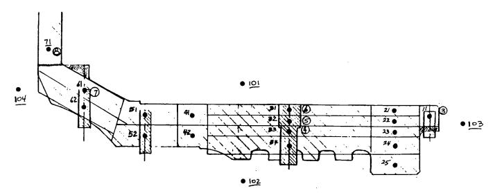
Figure 11. Finite element grid and boundary conditions for thermal model, GM 5307.
