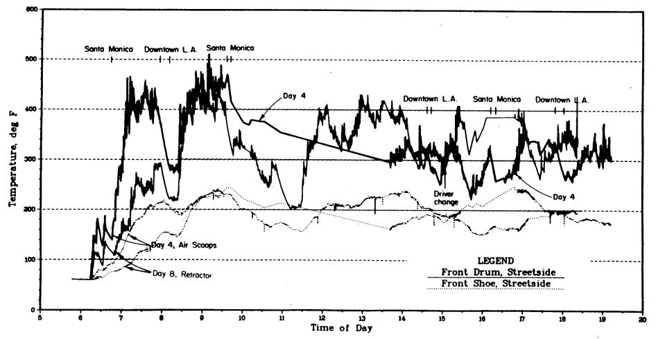
Figure 25. Front brake drum temperatures, with and without air scoop, 80/20 route.
