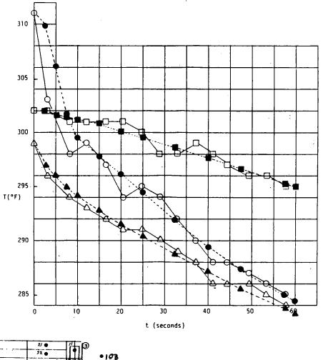
Figure 12. Final matched thermal conditions in front drum of GM 5307 bus.
