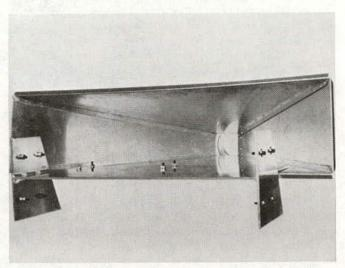
Figure 17. Air scoop designed to direct air flow across the front drum of an RTS-II ADB.
