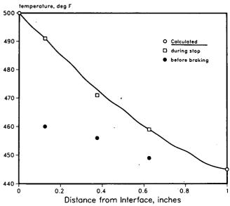
Figure 3. Brake drum temperatures measured before and during braking.
