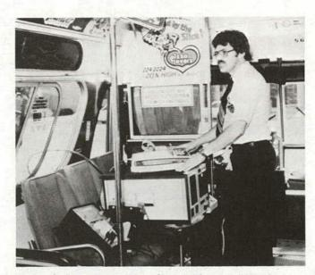
Figure 9. Data acquisition package in-place on COTA bus.
