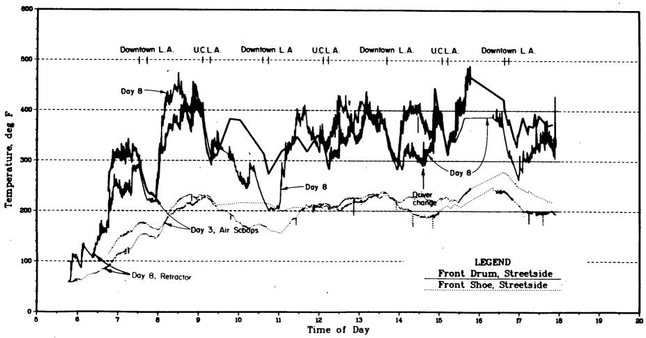
Figure 26. Front brake drum temperatures, with and without air scoops, 84/20 route.
