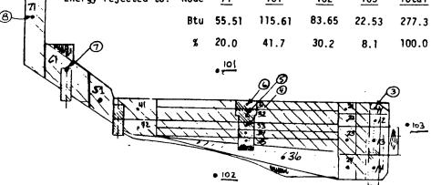
Figure 13. Final matched thermal conditions in front drum of GM RTS-II.
