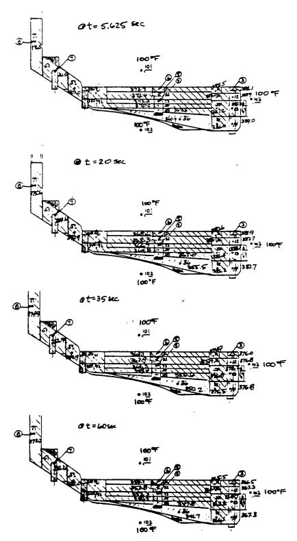
Figure 15. Temperature profile during cooling in front brake drum, GM RTS-II model.
