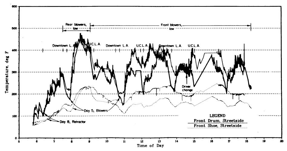
Figure 24. Front brake drum temperature, with and without blower units, 84/20 route.
