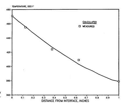
Figure 2. Drum temperature vs distance from drum/shoe interface during nonbraking time segment.
