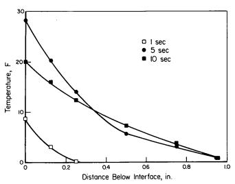
Figure 4. Temperature profiles in semiinfinite solid with constant heat flux (initial temperature = 0°F).
