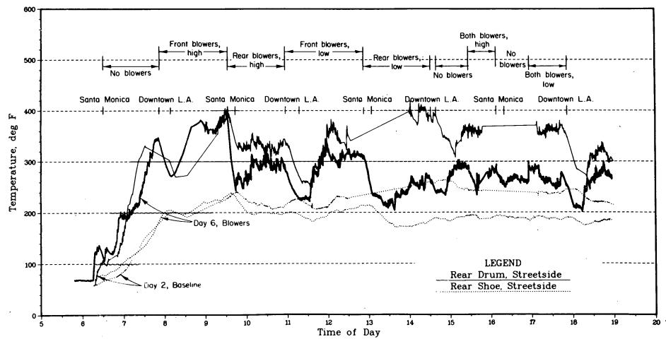
Figure 22. Rear brake drum temperatures, with and without electric blower units, 80/20 route.
