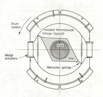
Figure 18. Schematic of retractor mechanism.
