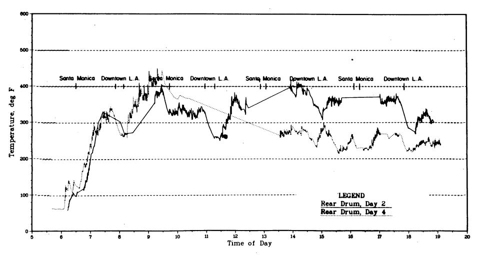
Figure 19. Near-surface brake drum temperature, GM RTS, 80/20 route (baseline temperatures for two separate days).
