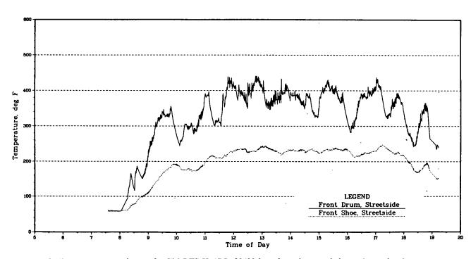
Figure B-2. Time-temperature history for GM RTS-II ADB, 80/20 line, front drum and shoe, asbestos-free linings.
