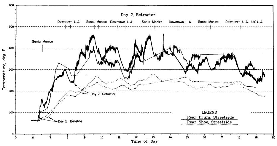
Figure 27. Rear brake drum temperature, with and without brake retractors, 80/20 route.
