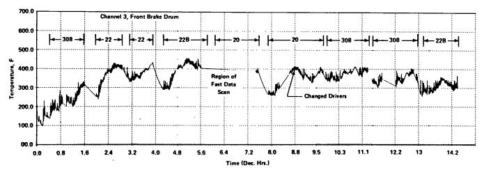
Figure B-1. Time-temperature history for GM RTS-II ADB, 83/20 line, front drum and shoe, asbestos-phenolic linings.
