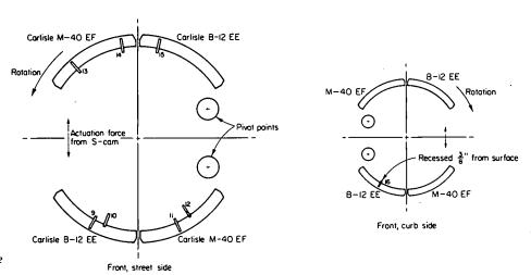
Figure 7. Location of front brake drum and brake shoe thermocouples, GM 5307 "New Look" bus, Phase I experiments.
