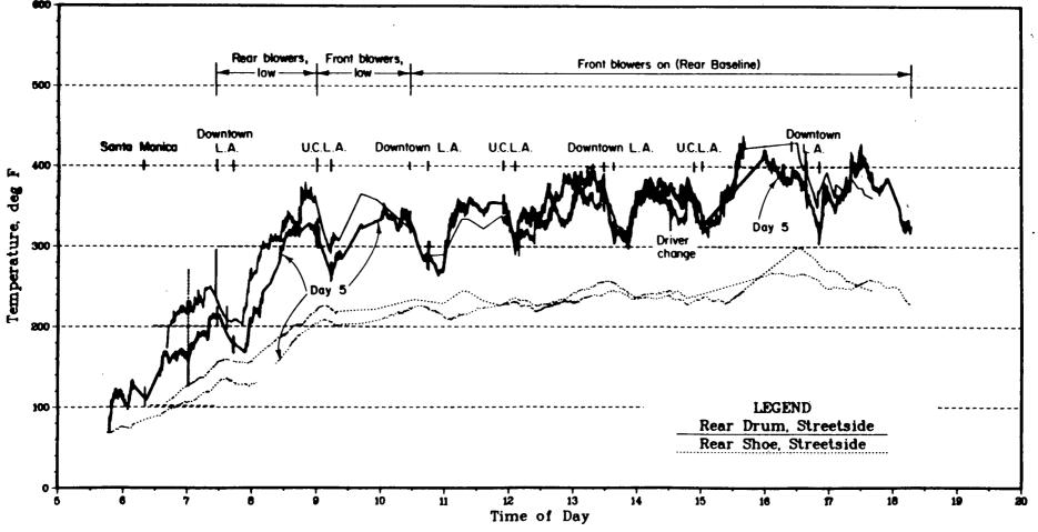
Figure 20. Near-surface brake drum temperature, GM-RTS, 84/20 route (baseline temperatures for two separate days).
