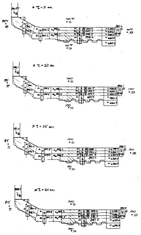
Figure 14. Temperature profile during cooling in front brake drum, GM 5307 model.
