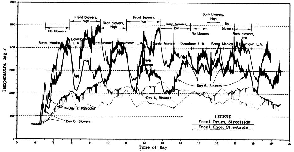
Figure 23. Front brake drum temperature, with and without blower units, 80/20 route.
