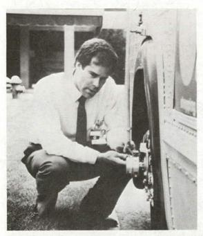
Figure 8. Slip ring assembly on front wheel of COTA bus.
