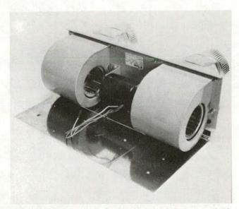
Figure 16. Blower units designed to direct cooling air across brake drums.
