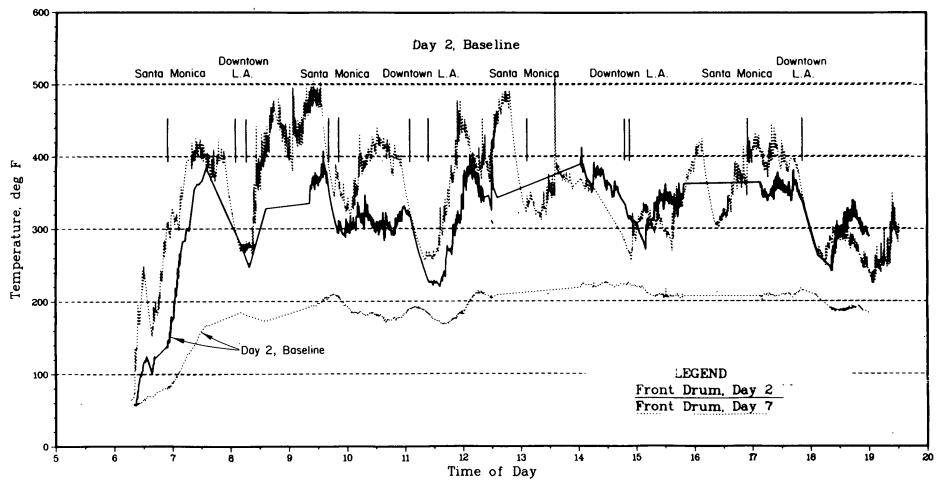
Figure 21. Front brake drum baseline temperature, GM-RTS, 80/20 route.
