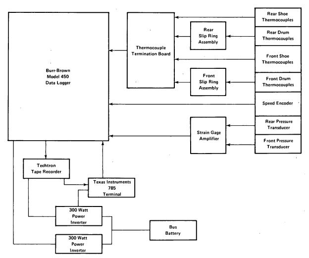
Figure 6. Block diagram of instrumentation.
