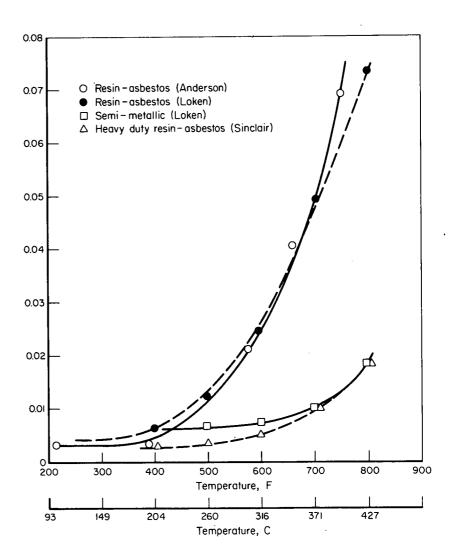
Figure 5. Wear-temperature relationship for selected brake material studies.
