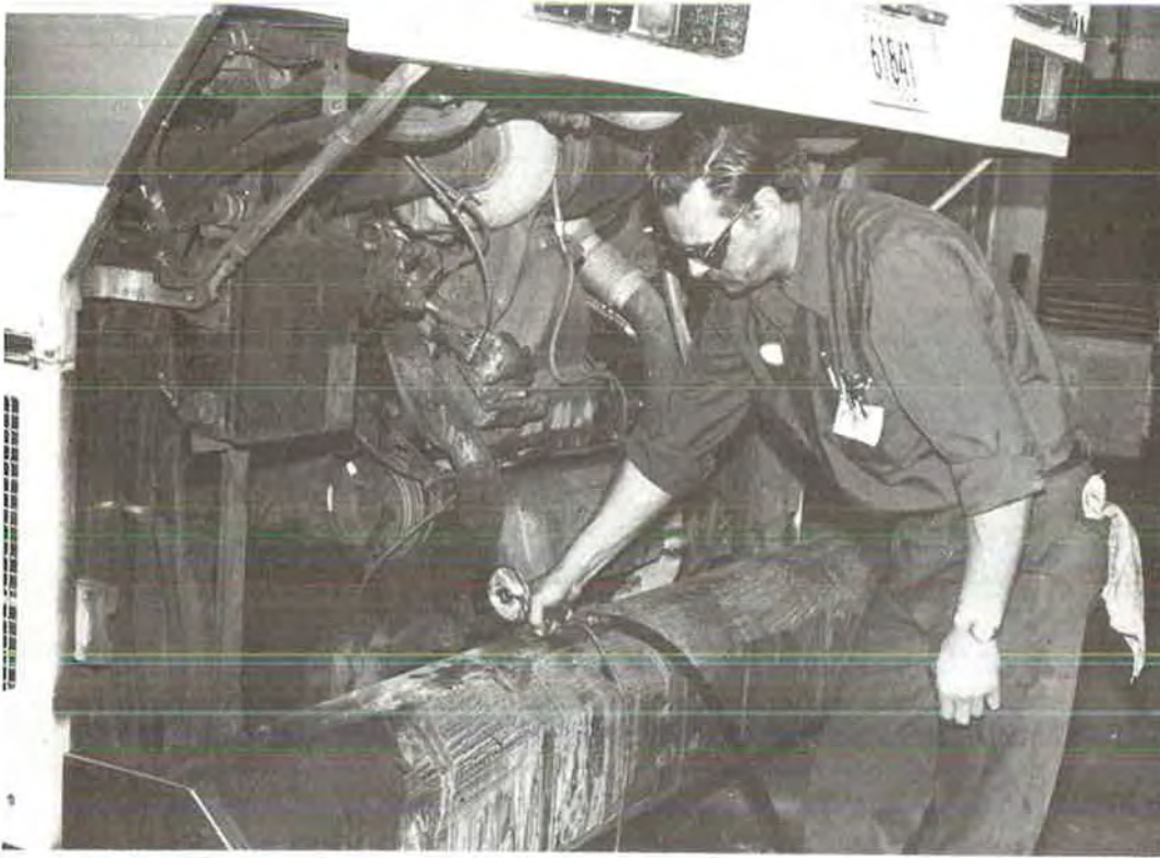
FIGURE 8 Adding engine oil with calibrated dispenser nozzle.
