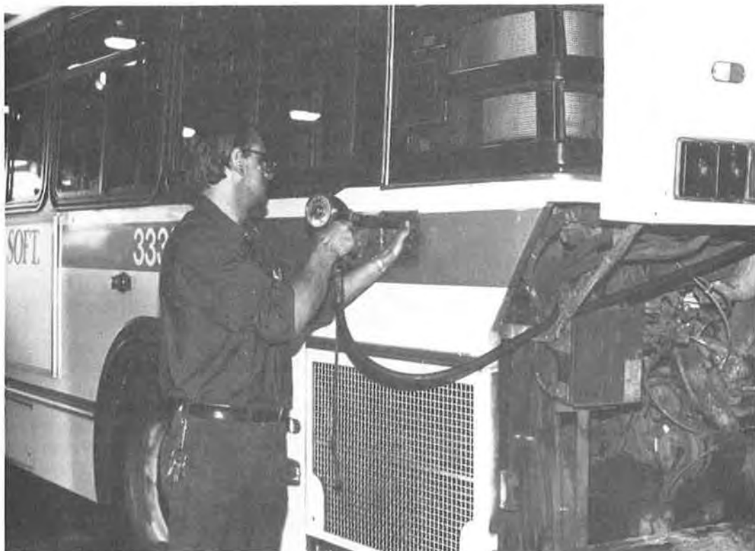
FIGURE 11 Inspector adding pre-mixed coolant with a calibrated dispenser nozzle.
