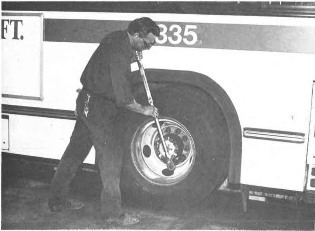
FIGURE 3 Inspector checking wheel nuts with torque wrench.
