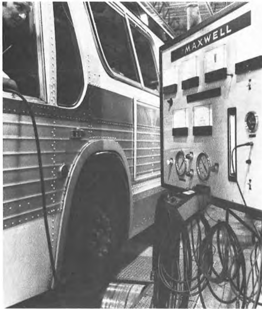
FIGURE 7 Mechanic checking front axle brakes, steering, and alignment as part of a 12-minute complete diagnostic check of both axles and power units with a combination chassis dynamometer/brake tester/high-speed road-test simulator.
