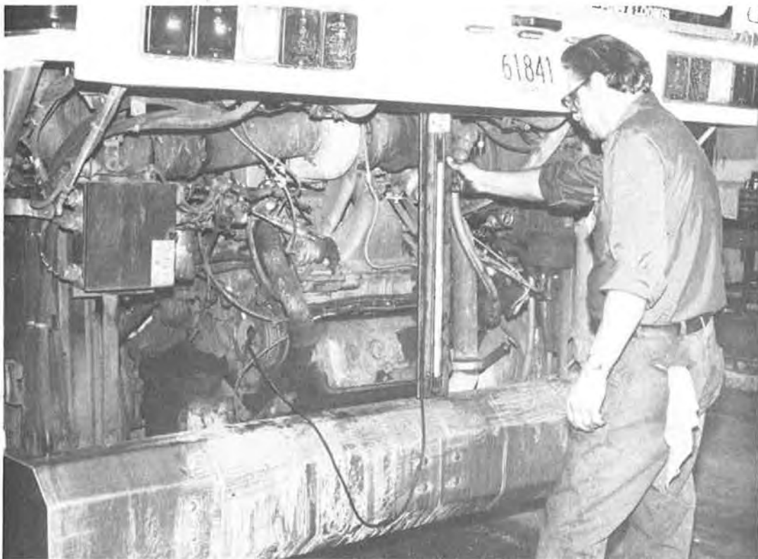
FIGURE 4 Mechanic checking air intake restriction with the manometer tube.
