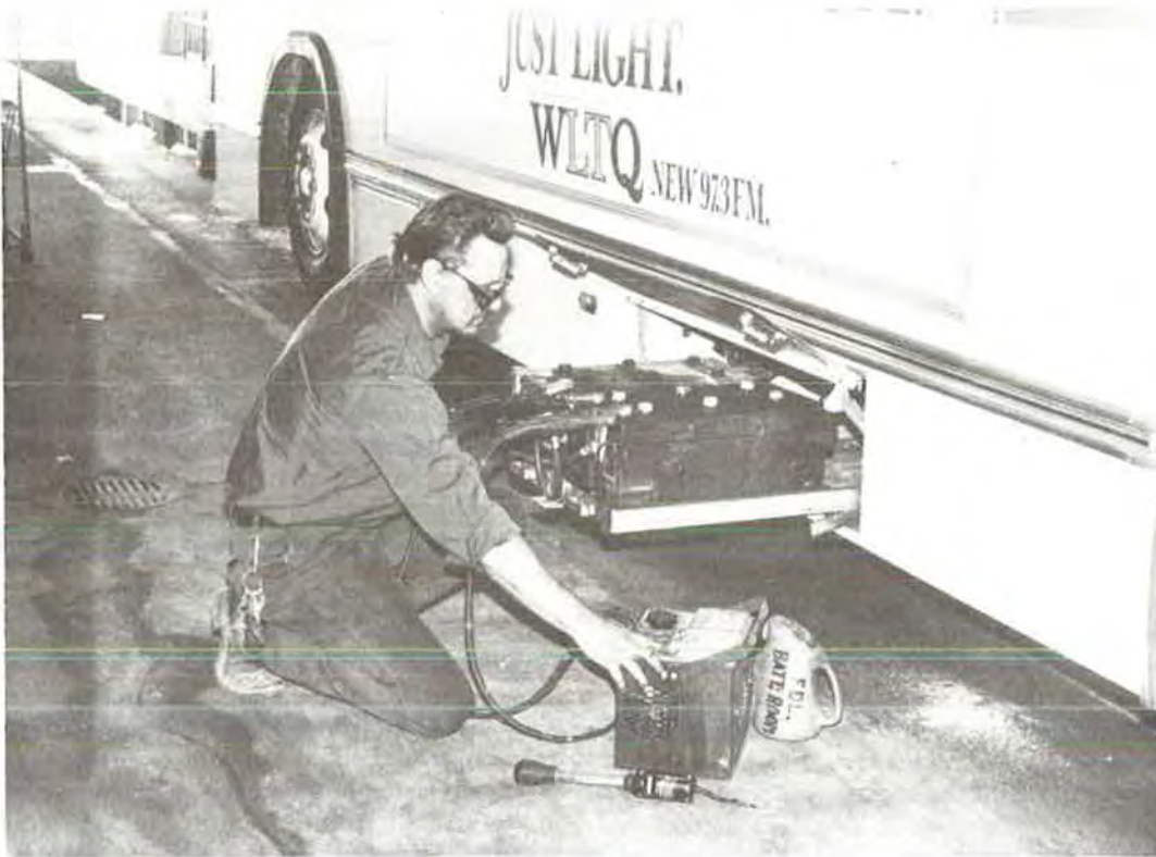
FIGURE 1 Battery condition check with hydrometer and ammeter-voltmeter tester along with container for distilled water.
