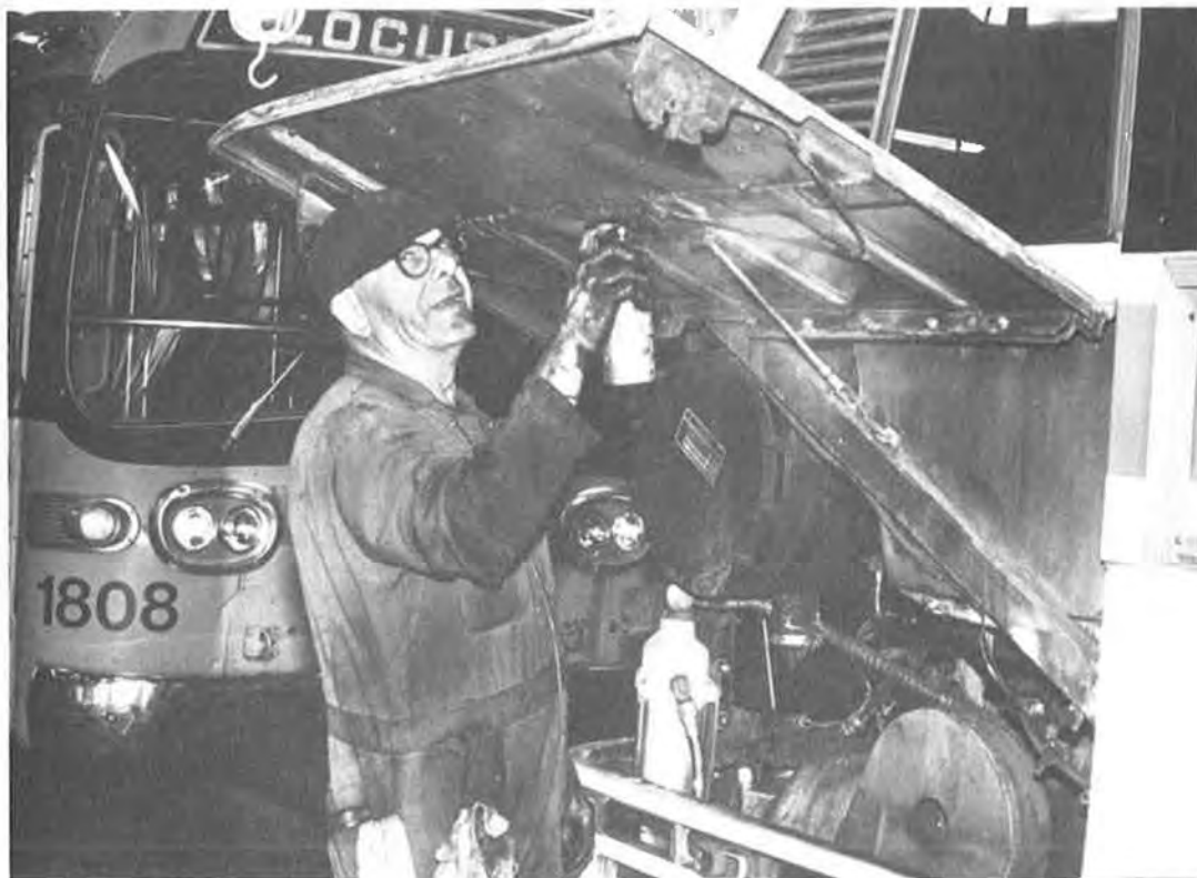
FIGURE 10 Lubrication of engine compartment door hinges with a spray oil dispenser.
