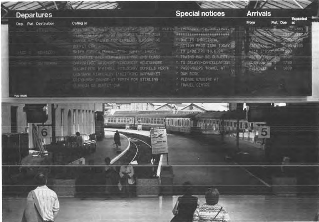
FIGURE 13 Flip dot changeable message sign at the Inverness, Scotland railroad station. (Photo courtesy of Vultron, Inc.)
