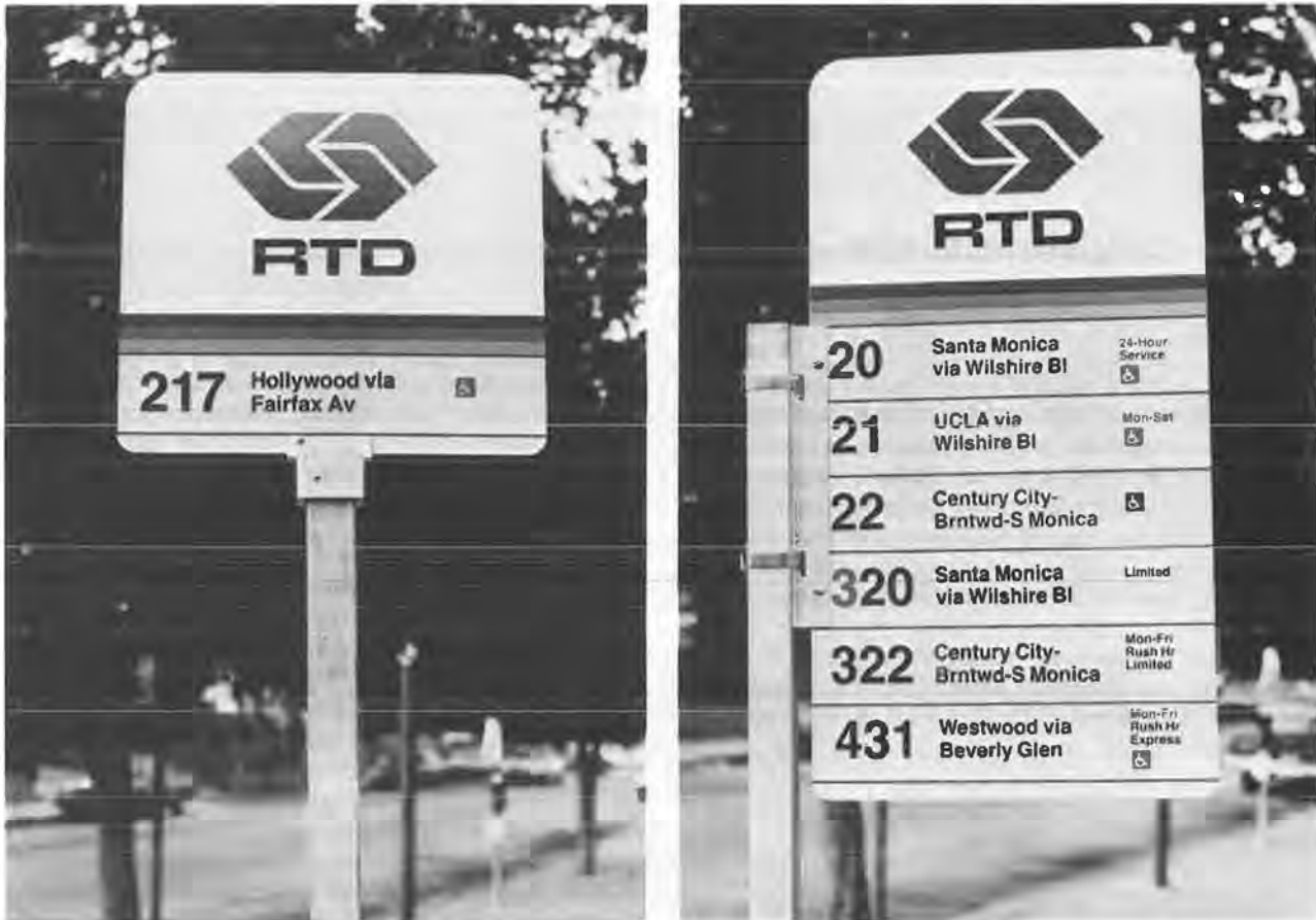
FIGURE 4 Southern California Rapid Transit District bus stop identification and modular bus route sign. (Photos courtesy of SCRTD.)
