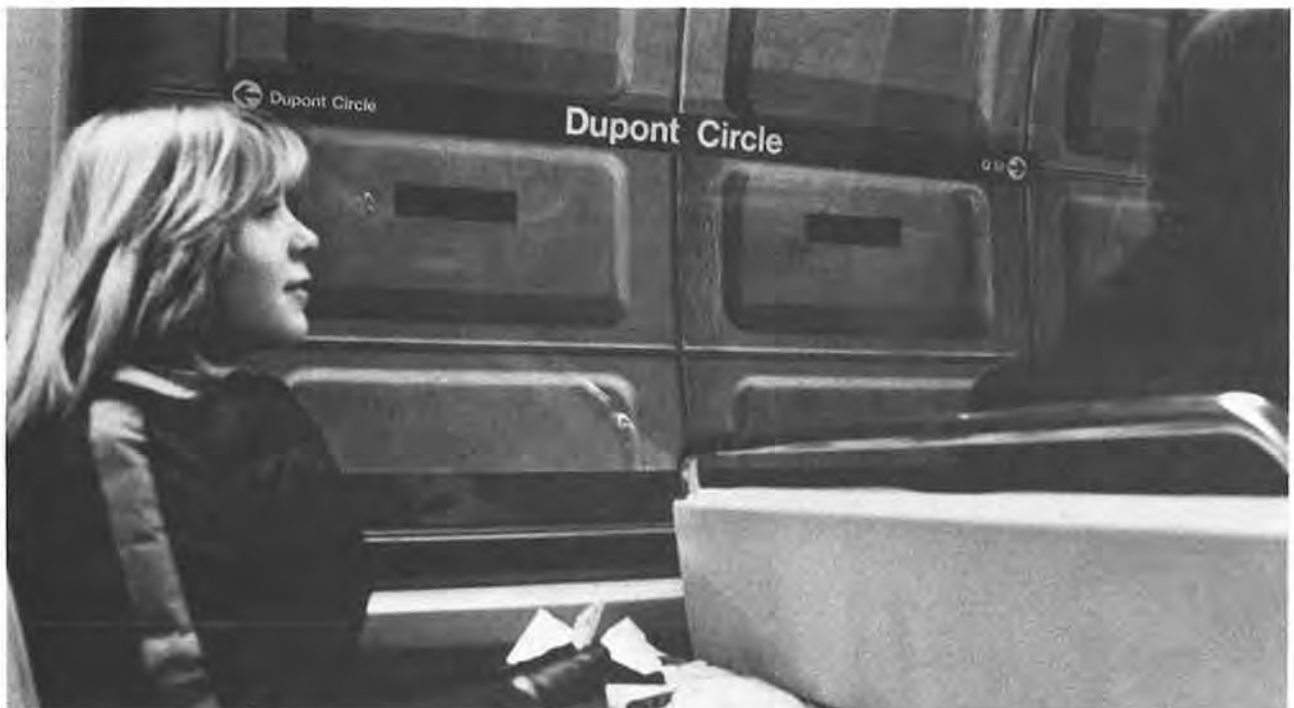
FIGURE 3 Station identification signing follows the continuity and repetition principles of communication, allowing passengers to confirm direction en-route by comparison with on-board route maps, or pocketmaps. (WMATA photo by Paul Myatt.)
