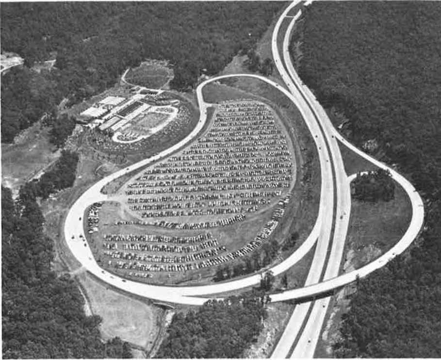
The Anthony Wayne Recreation Area on the Palisades Interstate Parkway, located some 40 miles north of New York City, is an example of the coordination of freeways with major recreation facilities. (Source: NCHRP Report 53.)
