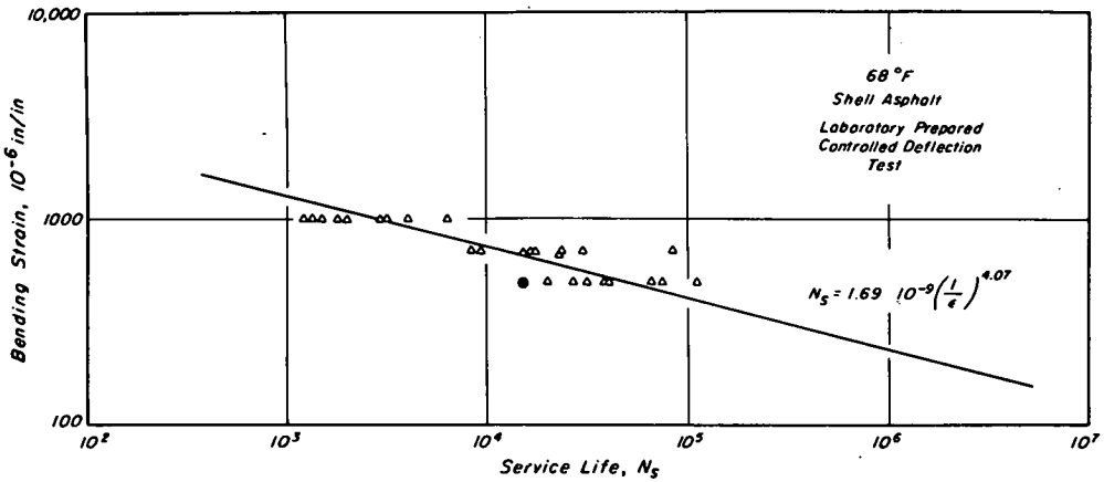
Figure 6. Initial bending strain versus service life in controlled-strain (deflection) tests on laboratory-prepared specimens.
