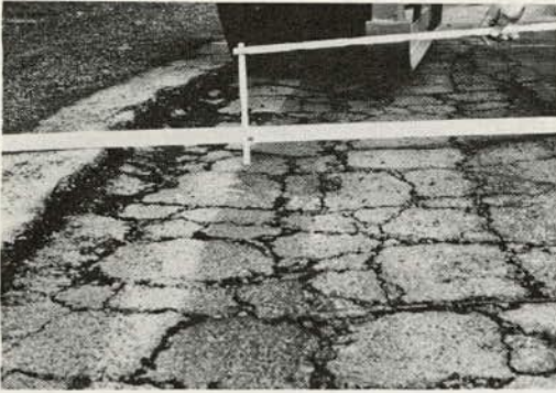
Figure 24. Well-developed crack system on underside of asphalt sections that showed little crack development at surface.
