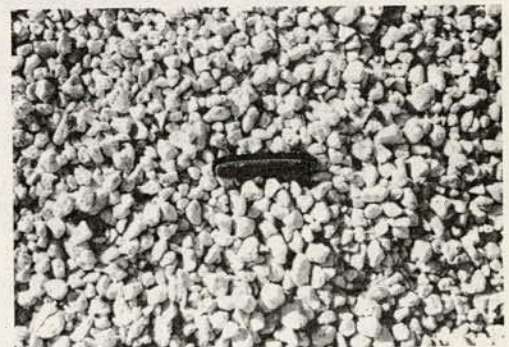
Figure 5. Three-quarter-in. aggregate used in fibrous concrete mix for Tampa overlay.
