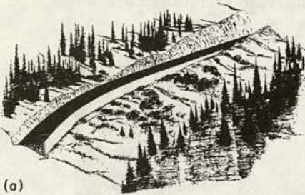
Figure 17. Artist's conception of (a) standard cantilever wall retaining a portion of I-90 near Snoqualmie Pass and (b) same location using a gabion wall.
