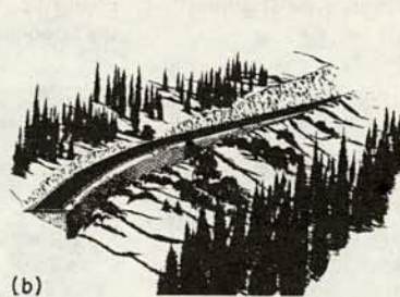
Figure 17. Artist's conception of (a) standard cantilever wall retaining a portion of I-90 near Snoqualmie Pass and (b) same location using a gabion wall.
