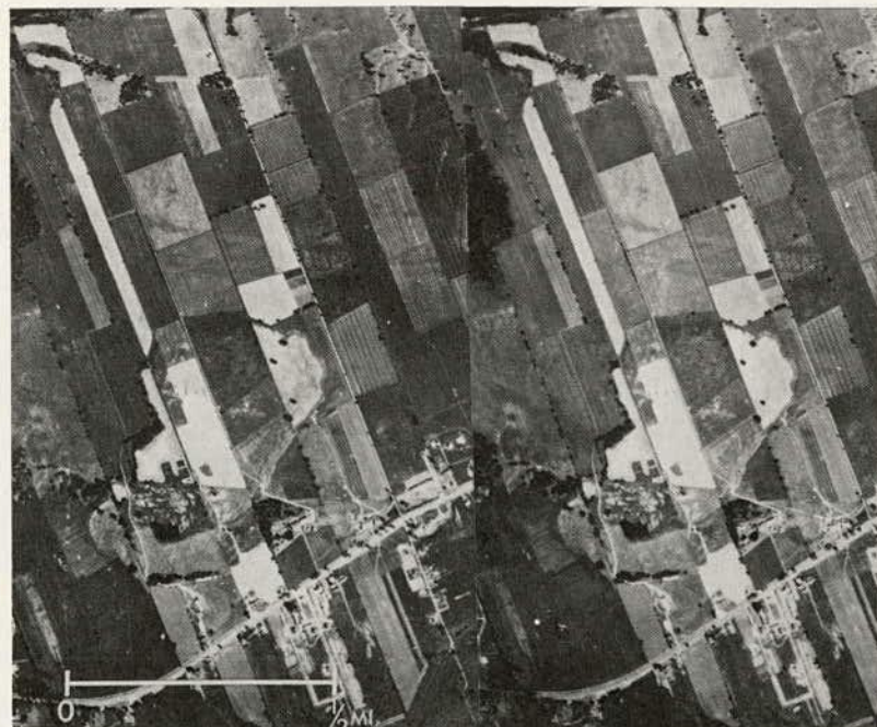
Figure 3.27. Example of earth flow in sensitive clays along Ottawa River east of Ottawa, Canada (3.17).
