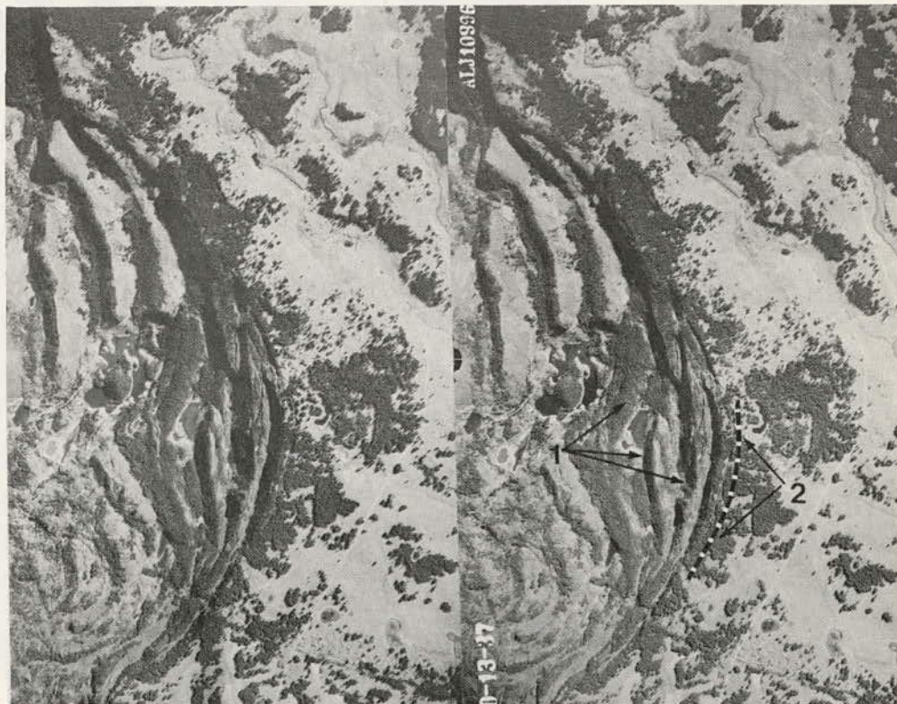
Figure 3.19. Basalt cap rock overlying impermeable shale deposits has resulted in massive landslides in Mesa County, Colorado. Large blocks of material have toppled and slumped off scarp face (1). Presence of incipient slide is indicated by cracks on crown of slide (2).
