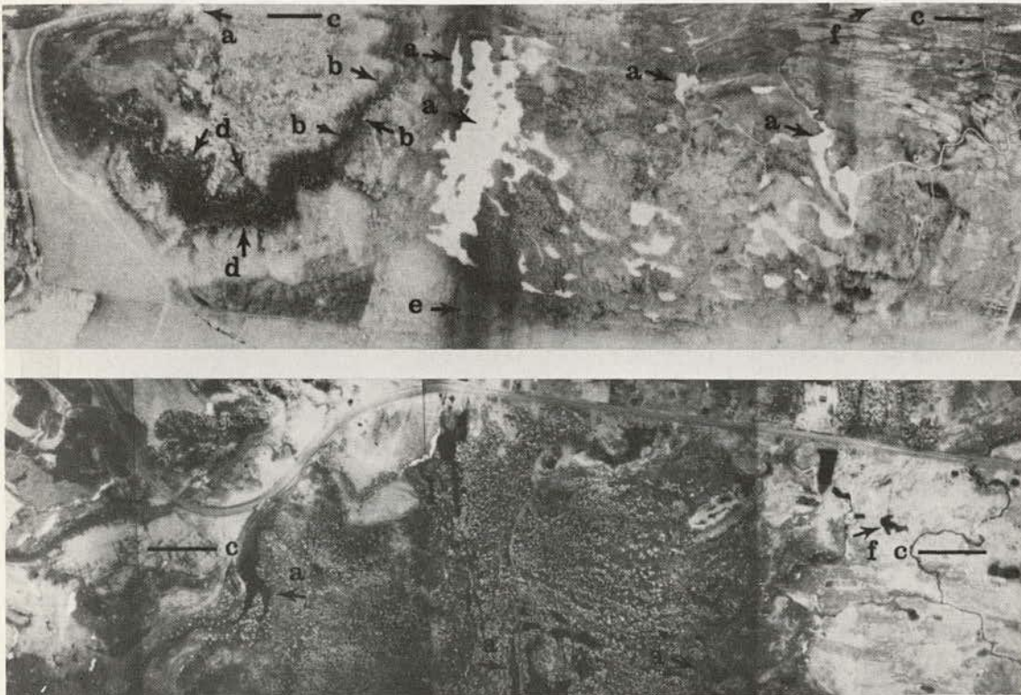
Figure 3.34. Predawn infrared imagery in 4 to 5- \mu m band (above) and mosaic prepared from black-and-white infrared photography (below) taken in Ontario, Canada (3.33). Line c-c represents common line on both images. Lettered areas are discussed in text.
