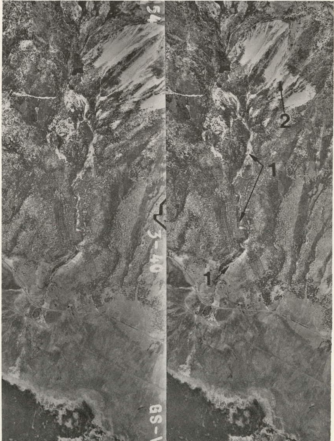
Figure 3.20. Large debris slide (1) with remnant scar (2) in granodiorite rocks on east front of Sierra Nevada Mountains just east of Lake Tahoe in Washoe County, Nevada. An estimated 95 Mm 3 (125 million yd 3 ) was involved; portions of toe of slide are buried under younger alluvium (3.36).
