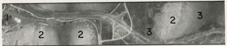
Figure 3.36. Nighttime infrared imagery of tilted sedimentary rocks in Schuylkill County, Pennsylvania. Lightest tones (1) are water or roads; next lightest (2) are shallow soils over continuous bedrock; medium gray tones (3) in bedrock area generally indicate more fractured rock and colluvial slopes.
