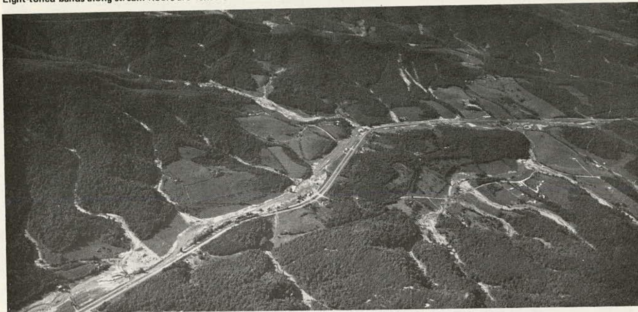
Figure 3.1. Catastrophic debris avalanches in Nelson County, Virginia, after torrential rains associated with hurricane Camille dumped 69 cm (27 in) of water August 19-20, 1969. Light-toned scars on tree-covered hillsides indicate locations of debris avalanches. Light-toned bands along stream floors are veneers of rubble and debris slide material.
