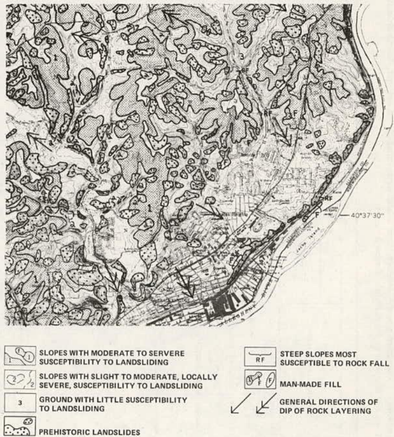
Figure 3.10. Portion of USGS Miscellaneous Field Studies Map MF-685B, Susceptibility to Landsliding, Allegheny County, Pennsylvania.
