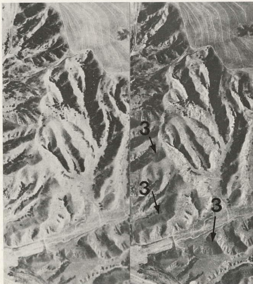
Figure 3.29. Cat steps can be seen on this enlarged section of area shown in Figure 3.28. Because of their small size, they appear as thin, wavy contours on hillside.
