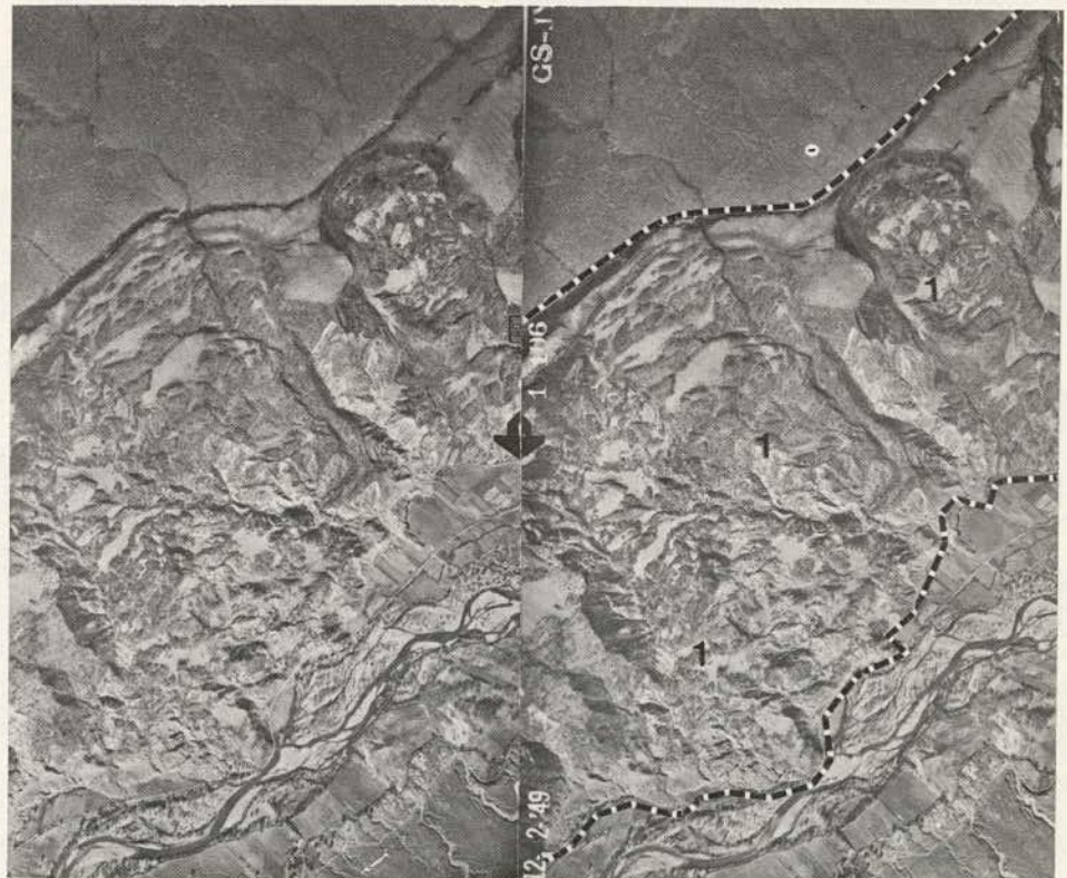
Figure 3.31. Old, massive landslide terrain in Rio Arriba County, New Mexico. Landslides (1) are of such magnitude that they are easily identifiable on common 1:20 000 aerial photographs as well as on smaller scaled photo-index sheets or even 1:1 000 000 satellite imagery (Figure 3.32). Most slides encountered in engineering projects are of smaller magnitude and difficult to identify at scales of 1:20 000.
