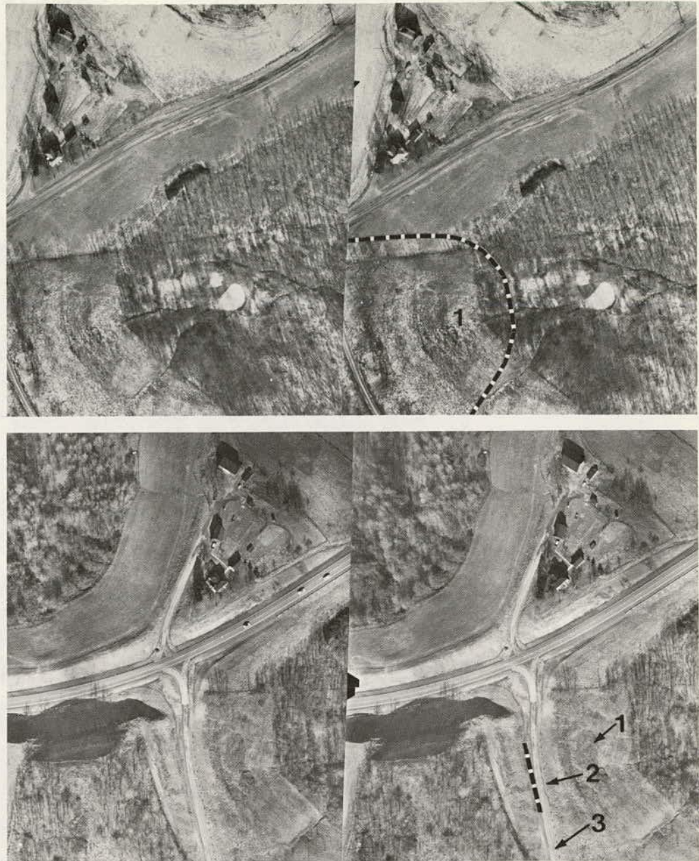
Figure 3.6. Before (top) and after (bottom) construction of Ohio-78 in Monroe County on unstable ground (3.22). Before construction, presence of hummocky ground (1) indicates unstable nature of terrain. Relocation of side road to meet new grade of highway placed side road on slide-prone slope, which resulted in small slide of embankment (2). Crack crossing road diagonally, seen as faint dark line (3), is site of possible future movement.
