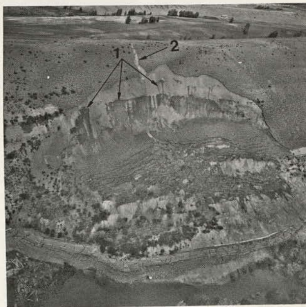
Figure 3.4. Oblique aerial view of extensive seepage zones (1) on scarp face of massive landslide in Kittitas County, Washington. Seepage was major cause of slide in these unconsolidated sediments. Remnant of dry sand flow (2) is seen above scarp face and is result of seepage at higher level. Landslide disrupted highway at base of slope and water canal carried through slope.
