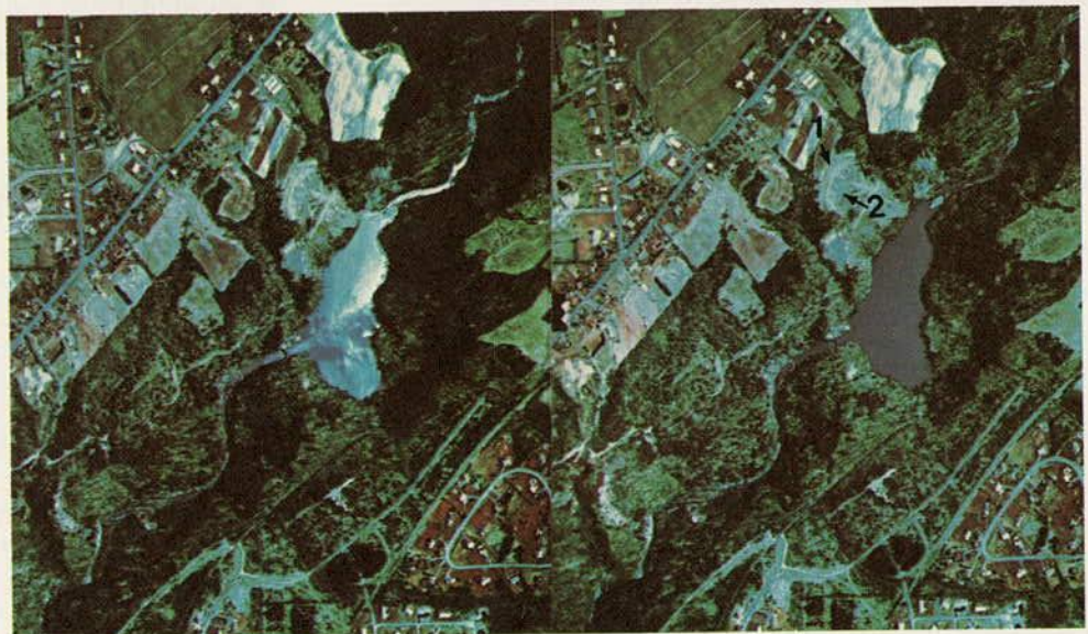
Plate 3.6. Color infrared photographs taken April 9, 1976, of area shown in Plate 3.4. Seepage zones and wet areas (2) are best seen on this film type. Dark tones are clearly distinct. It is too early for presence of luxurious vegetation, which could aid in delineating seepage areas. Boundary between two deposits is more distinct on this film than on black-and-white film, but contrast is not so sharp as on natural color film.
