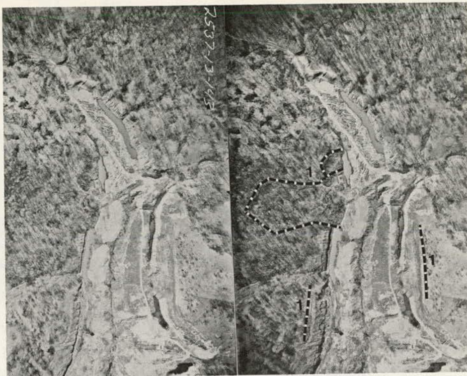
Figure 3.3. Slides (1) caused by undercutting of slopes by coal stripping operations in Washington County, Ohio (3.22).
