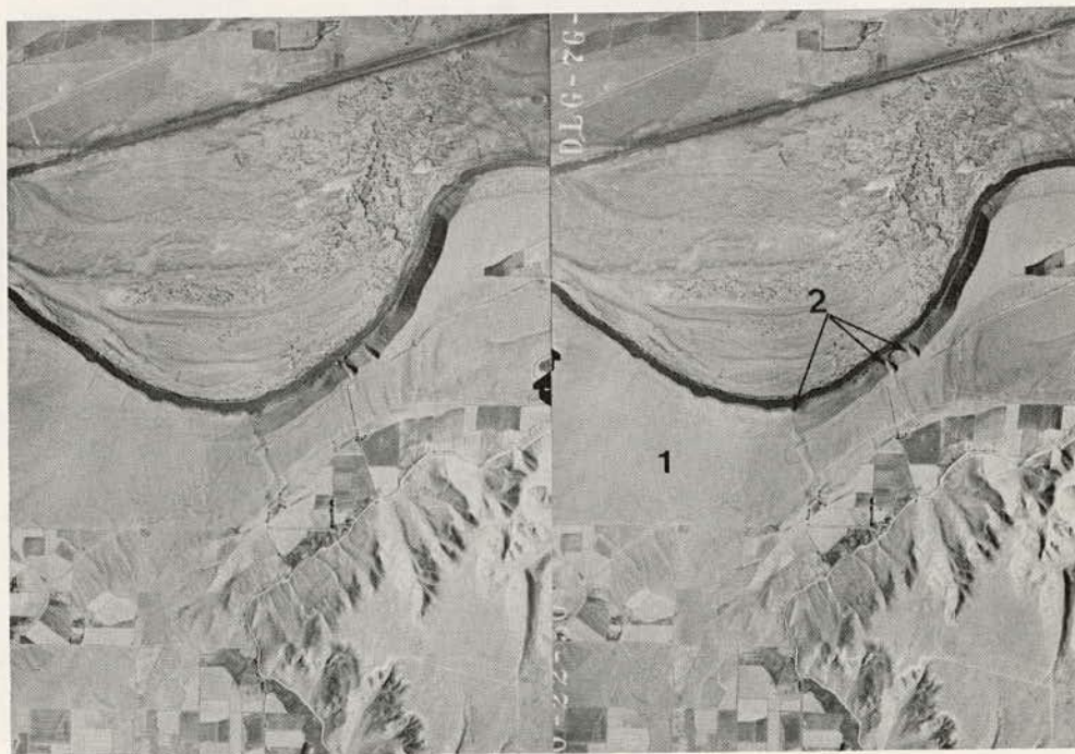
Figure 3.25. Sandy terrace (1) overlies basalt flow along Snake River in Elmore County, Idaho. Several dry sand flows (2) indicating sandy nature of materials are evident on terrace face.
