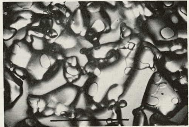
Figure 10. Dry snow grains in contact with a glass plate. Mirror-like contact plane surfaces are seen. Scale: 1mm.
