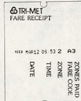
Ticket from Dispenser showing validation (Machine #, Date, Time, Zone Boarded, Fare Category, Zones Paid)
