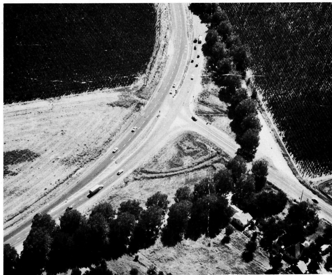
Figure 1. Channelized junction of local roadway (Howe Avenue) with curved section of main highway (Fair Oaks Boulevard). Note left-turn provision and well-organized wheel-track pattern shown on the pavement.
