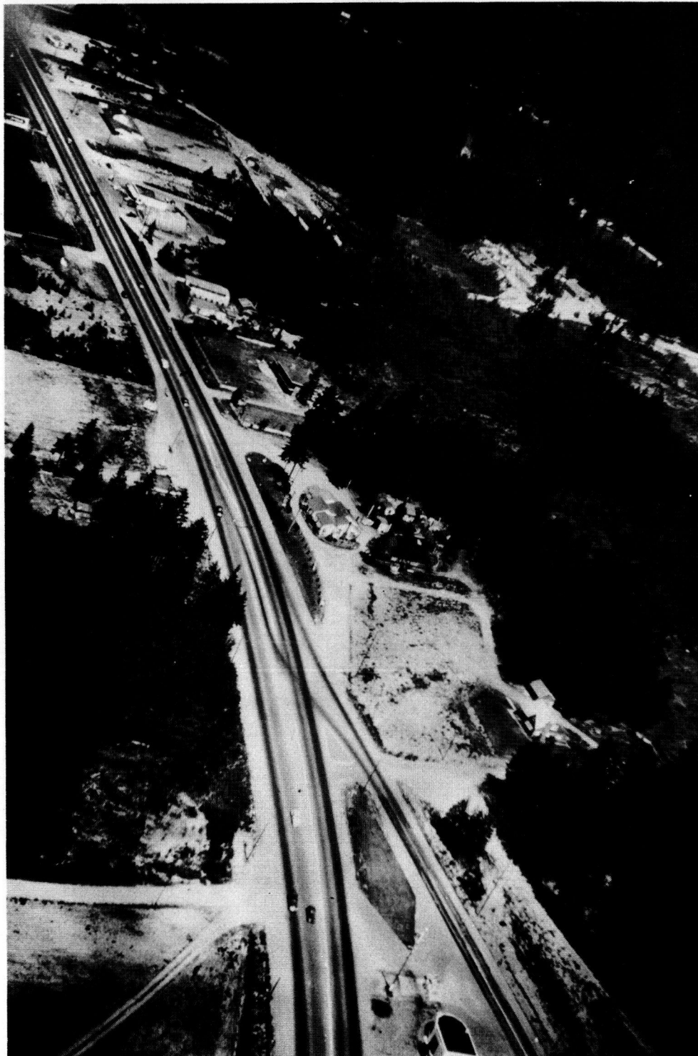
Figure 3. Channelization of Y-type intersection of 4-lane US 99 with 2-lane secondary road, State Highway 5-D, near Puyallup, Washington.
