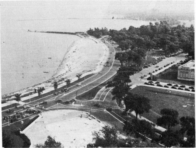
Figure 2. Traffic movement was measurably accelerated at the 57th Street intersection of Shore Drive after the installation of the center parkway (shown slightly to the right of center in the picture) and the application of well-defined lane marking. Removal of the old pavillion (from area in foreground) provided a clear view for southbound motorists. Shore Drive curves left along the shore of the lake, while North Circuit Drive is at the right.
