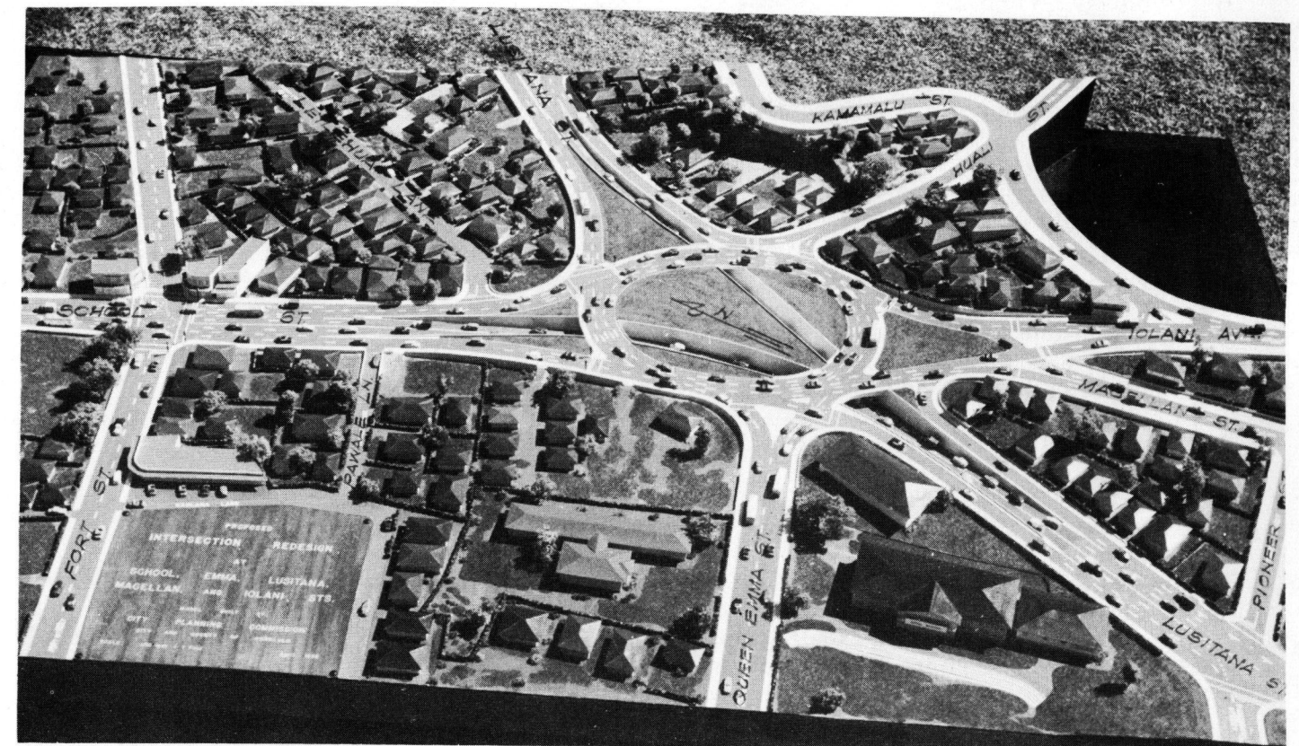
Figure 2. An excellent example of the use of a scale model to present a proposed intersection design. Note the fine detail and the clear presentation of a complicated reconstruction project. The cost of the model was $2,849.
