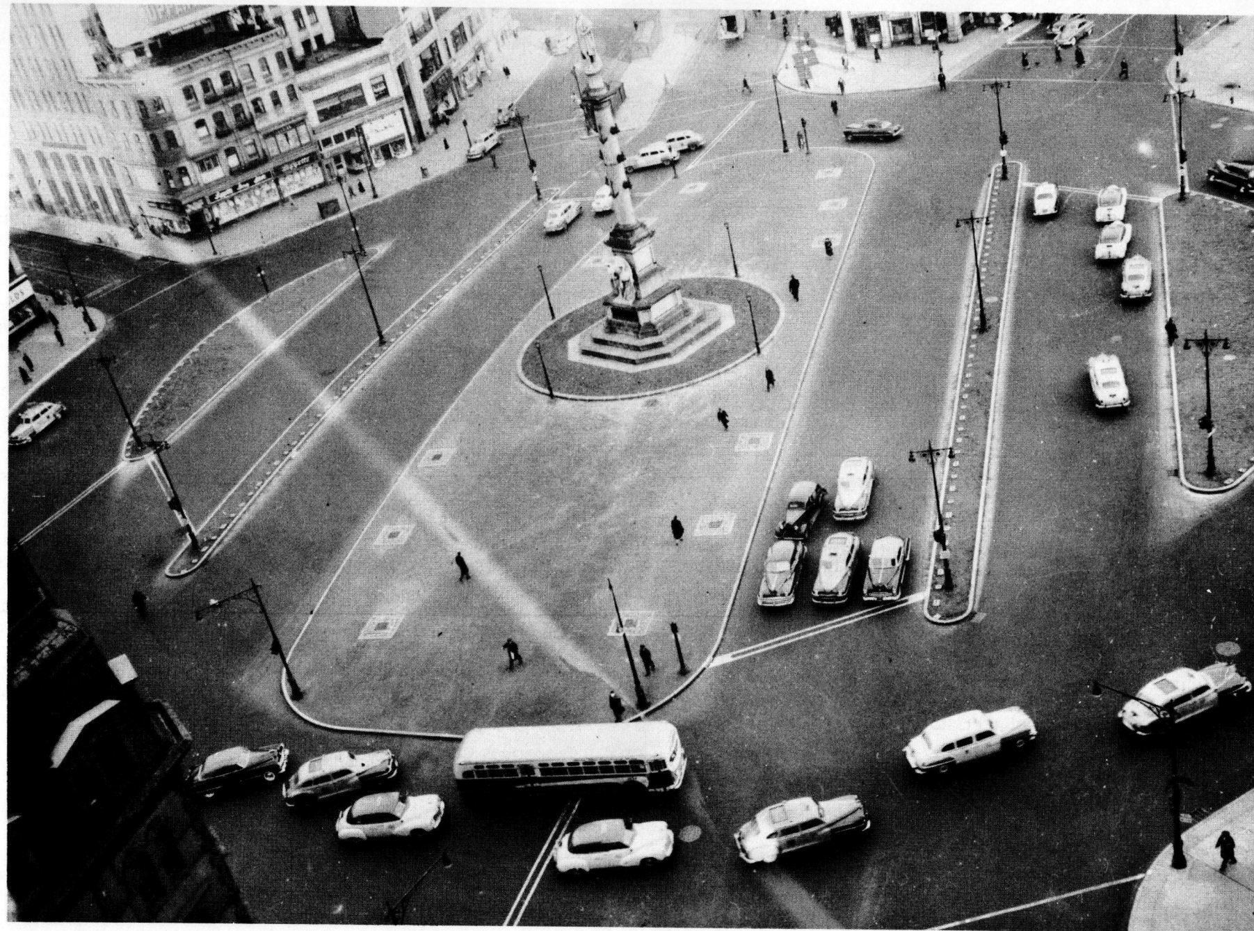
Figure 1. Revised intersection at Broadway and 8th Avenue, New York. All turning movements are made on periphery of original circle, with double through movements across center. Traffic signal control is necessarily complex.
