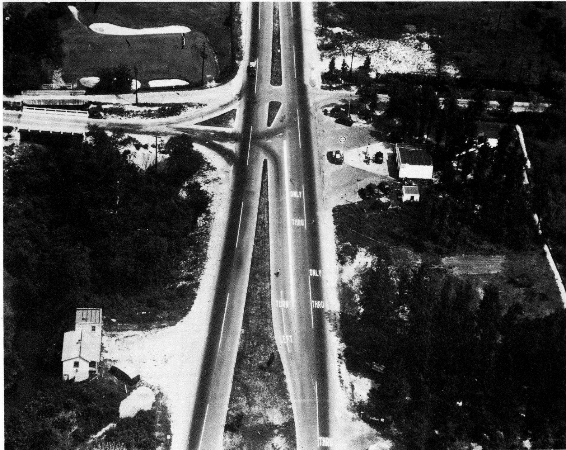
Figure 1. Four-way offset intersection of US 1 and Virginia 161 near Richmond. The wheel-track pattern shows excellent organization of traffic movements at intersection of a high-speed, heavy-volume artery with a secondary road.
