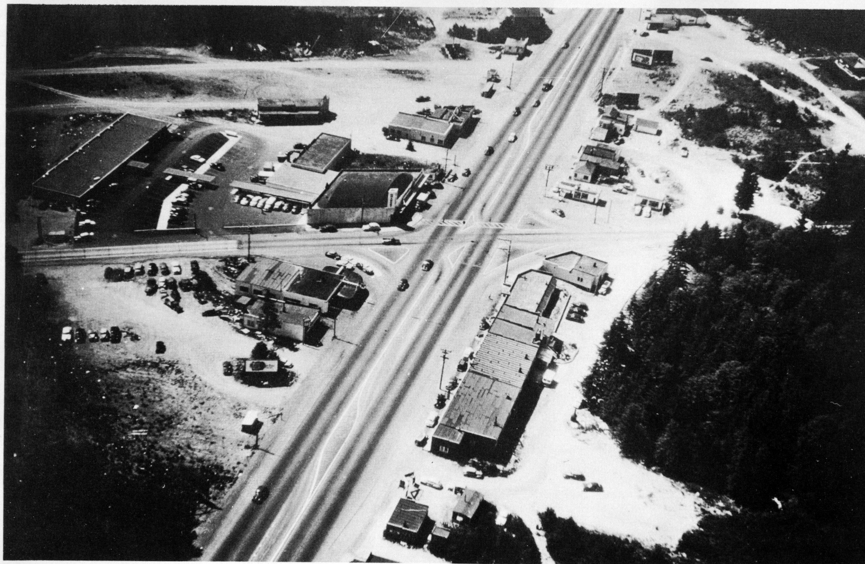
Figure 1. Aerial view of US 99 after 4-lane divided highway with 4-ft. median was widened, median expanded to include left-turn lanes, and channelizing islands added.
