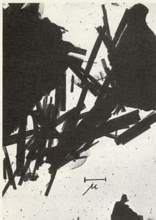
Figure 3. Cement exposed to humid \text{CO}_2 for 24 hr, then hydrated for 4 min immediately after the exposure; large crystals of ettringite have formed.
