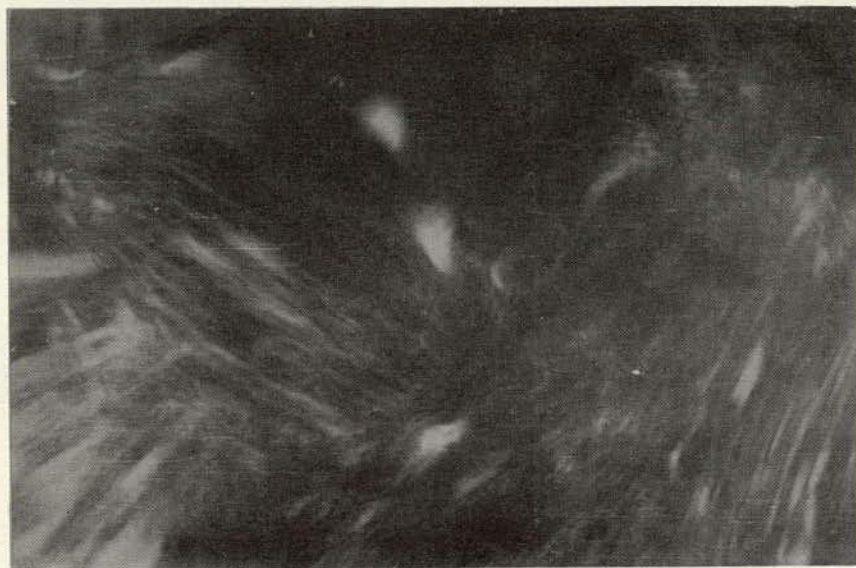
Figure 4. New formations of fibrous structure: Sample of commercial portland cement, w/c = 0.7 , 4 sec stirring; age is 6 min, magnified 1000 times.
