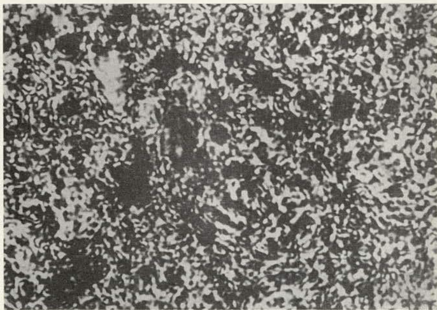
Figure 2. Thin microsection of cement stone from concrete after 20 years of normal hardening (microphoto, magnified 1000 times).
