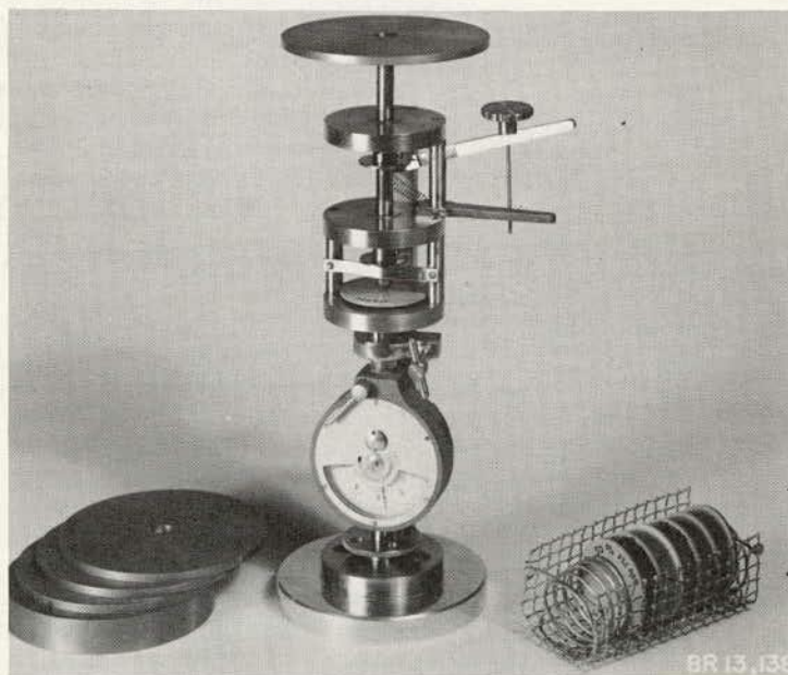
Figure 2(a). Miniature testing machine with dead weights for loading used for determining Young's modulus.
