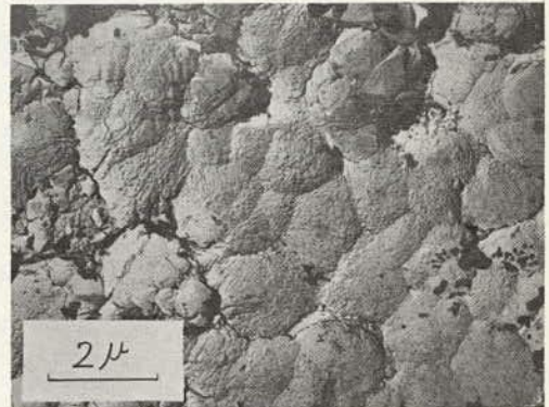
Figure 8. Electron micrograph of plazolite formed in the hardened blast-furnace slag powder.
