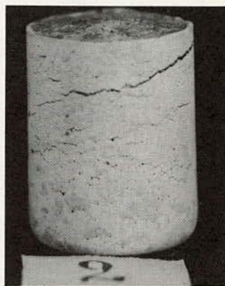
Figure 13. Cracking in concrete due to rapid heating.
