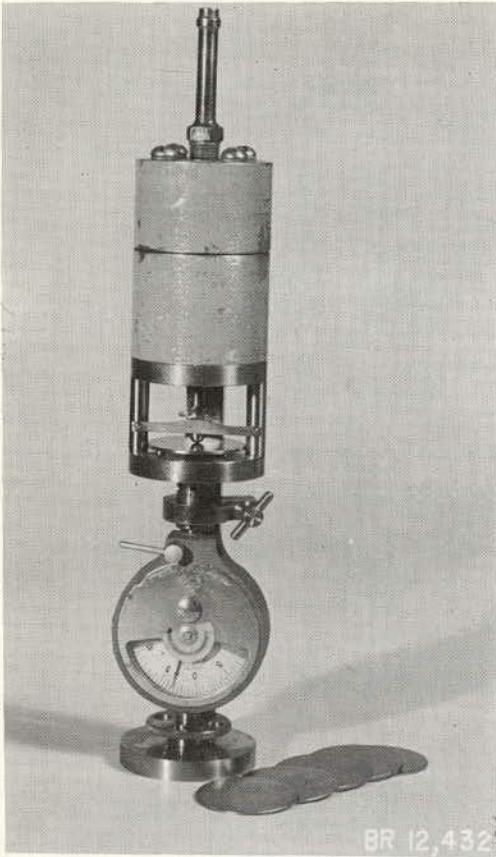
Figure 2(b). Miniature testing machine equipped with bellows for loading with air pressure, used for determining strength.
