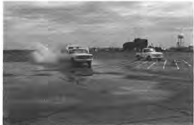
FIGURE 3 Puddles used in short-duration hydroplaning tests.
