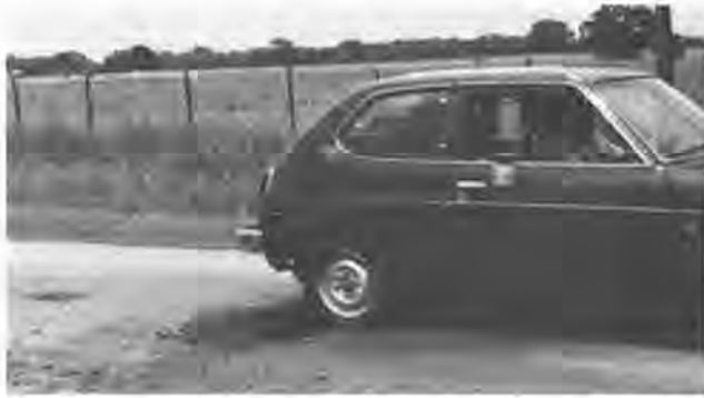
FIGURE 4 1978 Honda CVCC traversing hole 40 in. deep and 8 in. long.
