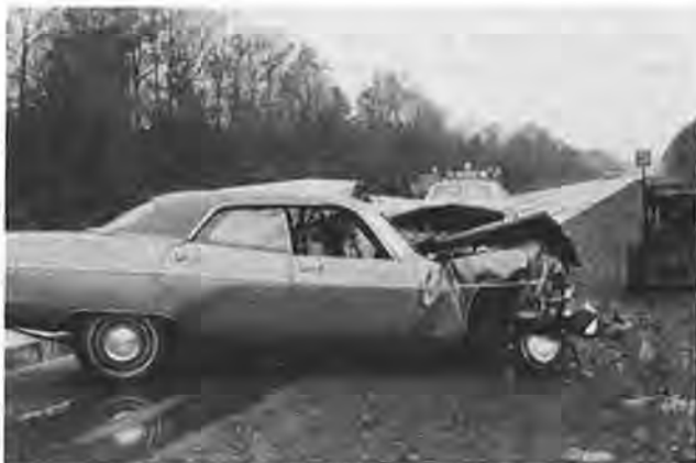
FIGURE 2 Result of excess speed and dynamic hydroplaning on flooded wheel paths.
