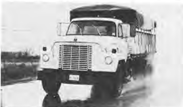
FIGURE 5 Contrast between spray caused by vehicles (4)--top: open-textured (porous) surface; bottom: conventional (nonporous) surface.
