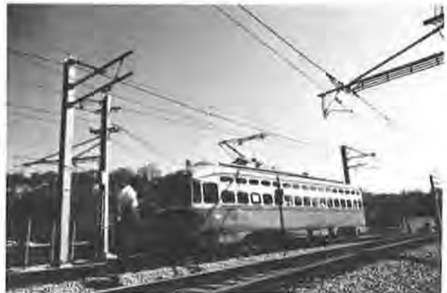
FIGURE 2 PCC car on new catenary system.
