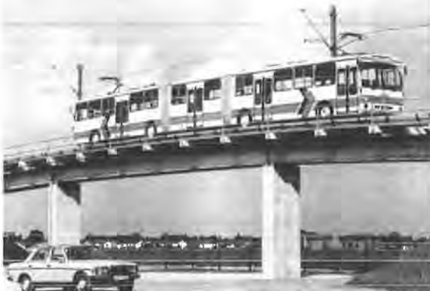
FIGURE 4 High-capacity bus on elevated track.
