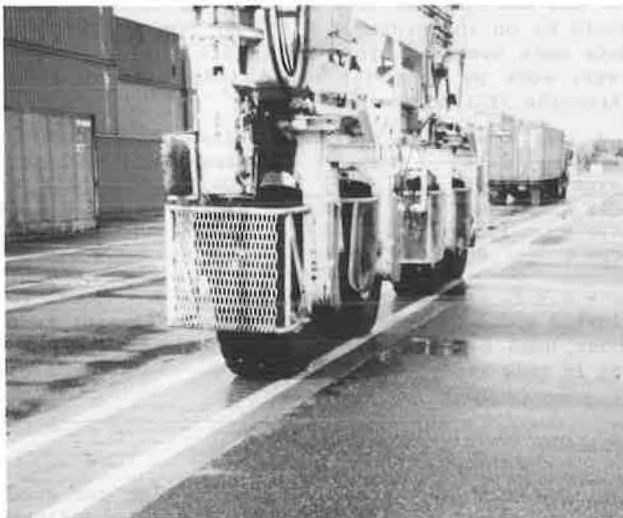
FIGURE 6 Gantry cranes operating on PCC slab.
