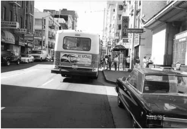
Figure A-23. Bus bulb on Stockton Street.
