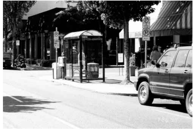
Figure A-51. “Crowding” at bulb for lift deployment.
