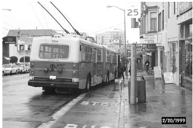
Figure A-8. Bus partially pulls into bus stop to avoid bus re-entry problem.
