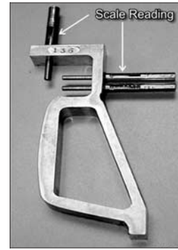
Figure 3.5. Measuring gage for AREMA 136 RE rails.
