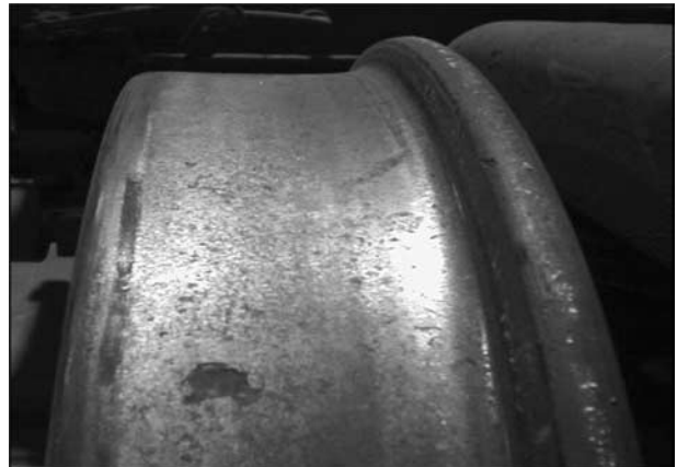
Figure A3-1. SEPTA cylindrical wheel wears into slightly hollow but stable shape on Suburban Route 101, LRV.
