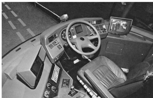
Photo 6-U. BRT vehicle with a video camera on the vehicle dashboard and painted, dashed lines on the pavement as key components of the optical guidance system.
