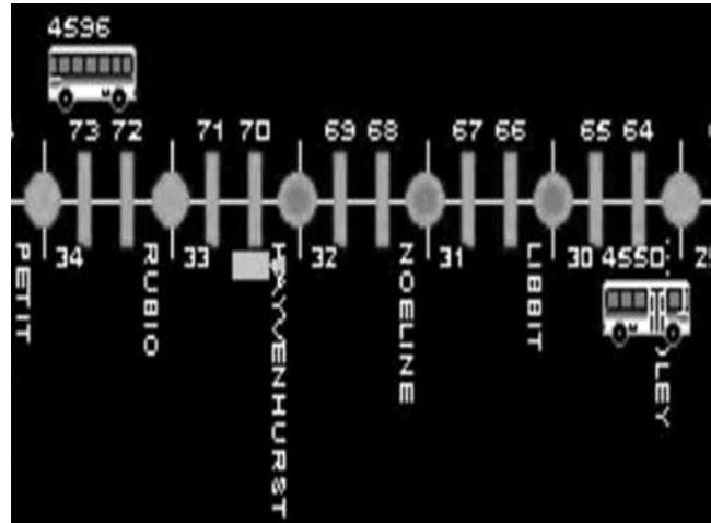
Photo 7-F. Control room bus location bus plan displays, Metro Rapid, Los Angeles.
