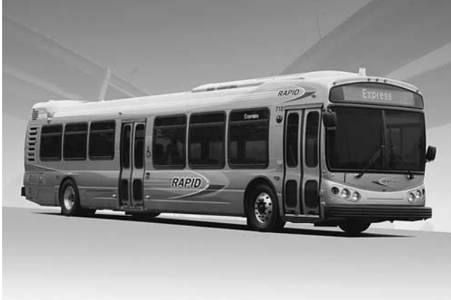
Photo 6-D. Composite 13.8-meter (45-foot) low-floor bus.
