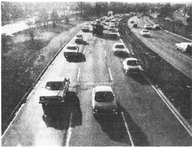
Illustration 1.1 Note the formation of large gaps in front of slow-moving trucks climbing the upgrade.
