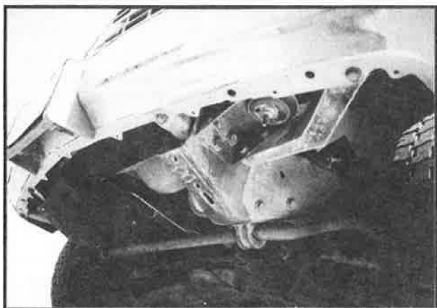
FIGURE 3 1989 Chevrolet 2500 front bumper reinforcement.
