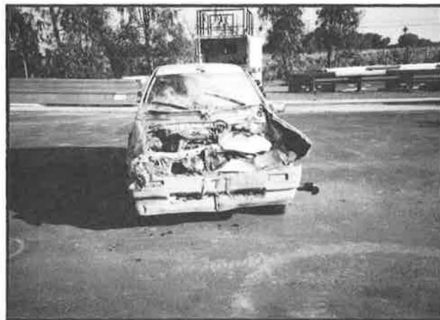
FIGURE 21 1988 Ford Festiva with missing hood after impact into inertial barrel array.
