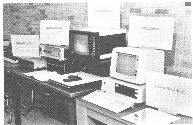
FIGURE 2 Microcomputer-controlled viewing system with high-resolution graphics capability.
