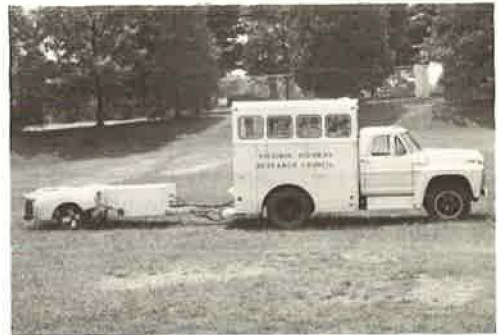
Figure 10. The Virginia Highway Research Council's skid-resistance measurement vehicle.
