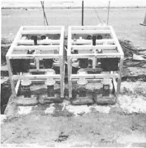
Figure 5. Microwave applicator modules.
