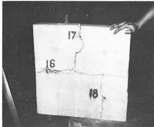
Figure 12. Results of three water-jet shots on microwave-cracked concrete.
