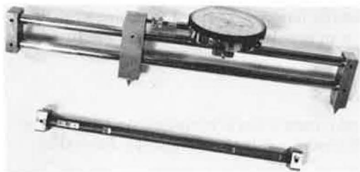
Figure 7. Extensometer and standard used for crack measurements.
