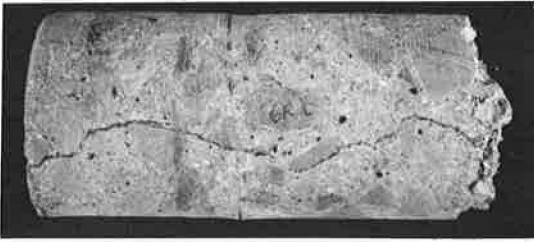
Figure 4. Left side view of core 6 showing continuous crack through core.
