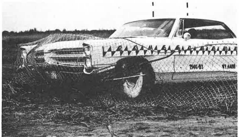
Figure 9. Vehicle entrapped in net after test D3.
