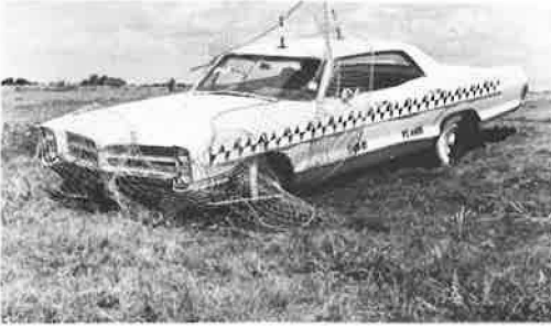
Figure 4. Vehicle after test D1 in which both tapes failed.
