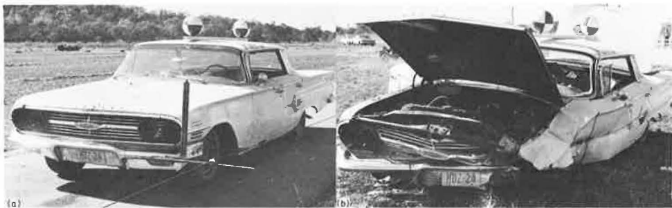
Figure 4. AA-5 test vehicle (a) before and (b) after impact.
