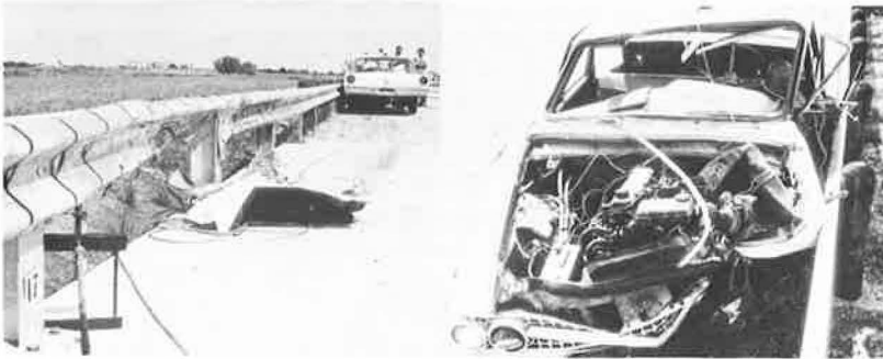
Figure 2. Barrier and vehicle damage after test T1-B.
