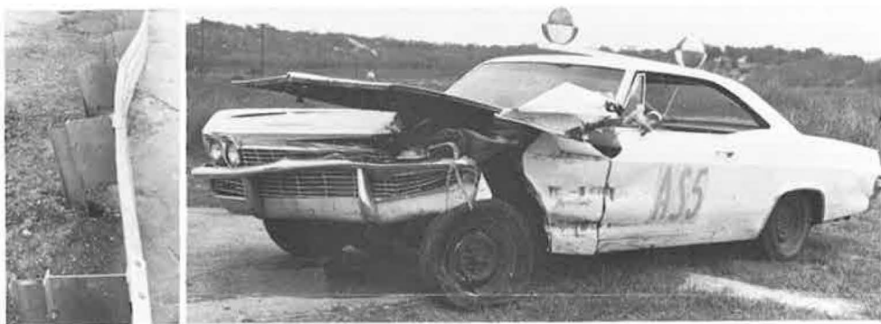
Figure 19. Beam and vehicle damage after test AS-5.
