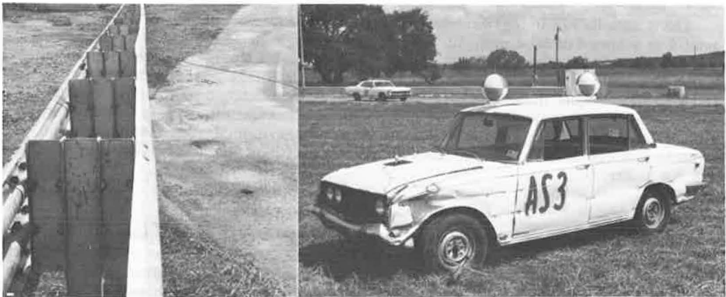
Figure 15. Beam and vehicle damage after test AS-3.
