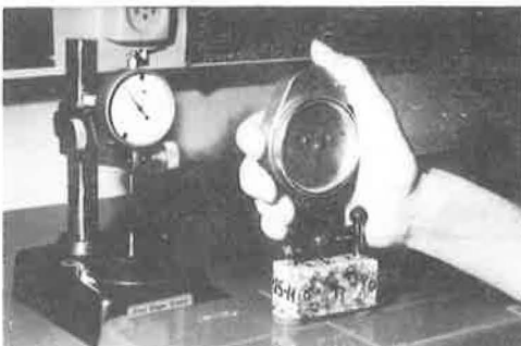
Figure 24. Measuring axial length L.
