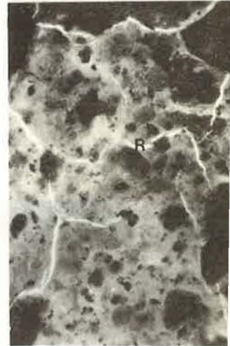
Figure 12. Concrete with cracks caused by frost damage (x50.3).
