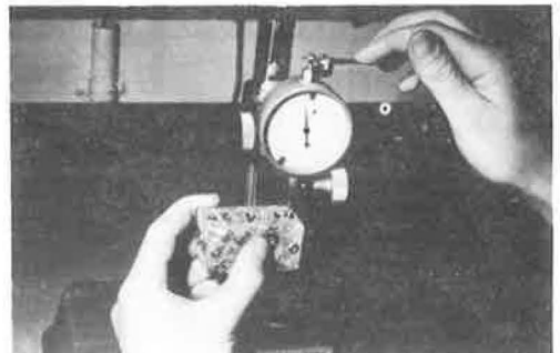
Figure 25. Measuring transverse length of Q perpendicular to prism's axis.
