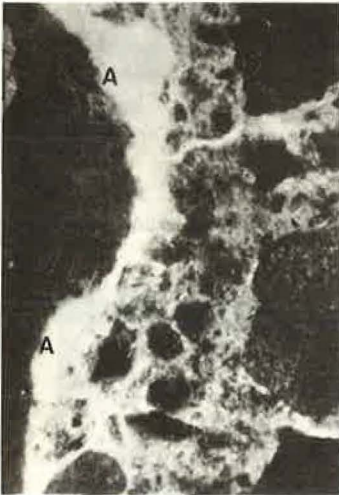
Figure 10. Concrete with disturbed adherence caused by high capillarity (x50.3).
