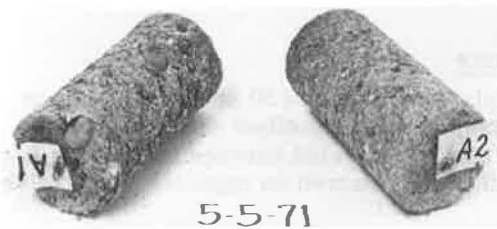
Figure 2. Concrete cylinders after 40 cycles in a sodium chloride solution.
