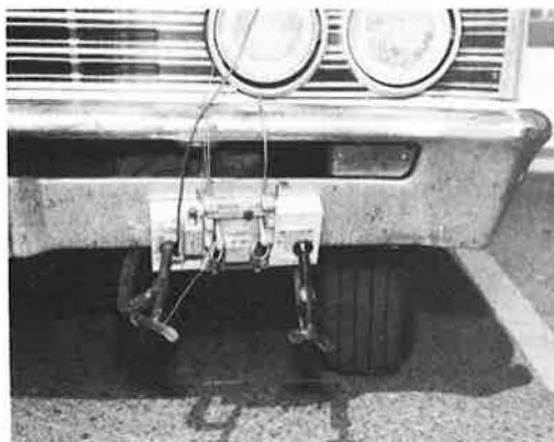
Figure 7. Two-shot marking device mounted on test vehicle.
