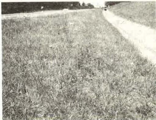
Figure 9. Same test area as shown in Figure 1 photographed in July 1972, approximately 2 years after spraying with varying rates of the picloram-2, 4-D combination herbicide. Even though the area was recently mowed, growth of wild carrot, buckhorn plantain, and other weeds was evident in the control plot in the foreground. The treated plots remained free of weeds.
