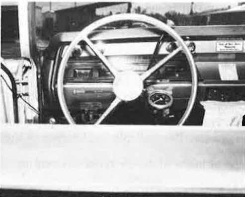
Figure 6. Special speedometer mounted adjacent to the steering wheel to better control the 10-mph test speed.
