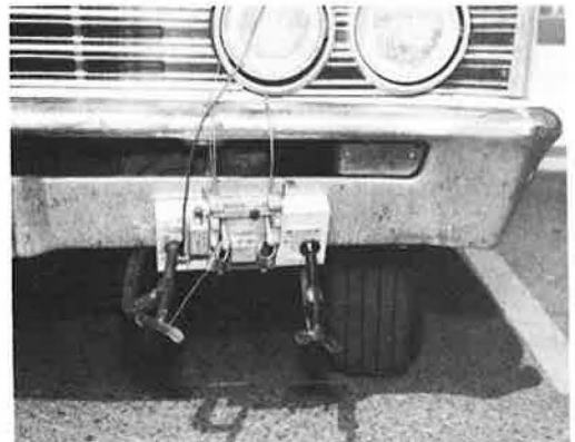
Figure 7. Two-shot marking device mounted on test vehicle.
