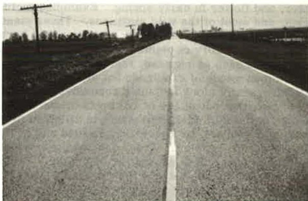
Figure 5. Portion of US-421 north of Lafayette, Indiana, in White County. The right side of the road received a single fall application of experimental formulation M-3766 (3 parts picloram and 1 part 2,4-D) at a rate of 2 lb active ingredient per acre. The left side of the road was unsprayed. Photographed in the spring following application.
