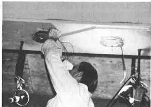
Figure 6. Strain gauge application.
