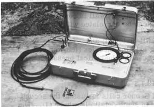
Figure 1. Terra Tec cell and readout device.
