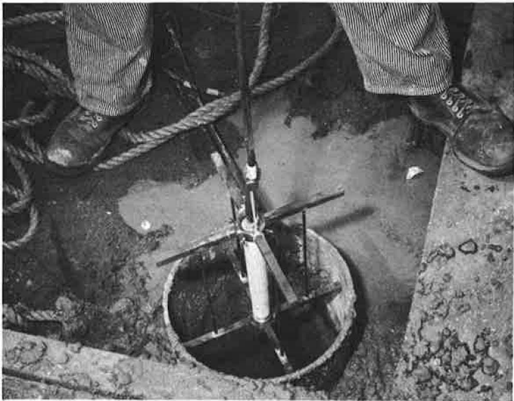
Figure 3. Installing strain meter and positioning bracket.
