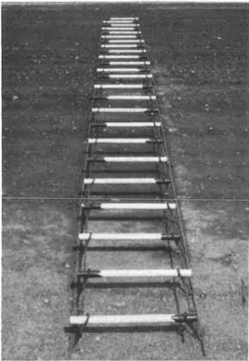
Figure 6. Bare dowel ends painted with red lead.
