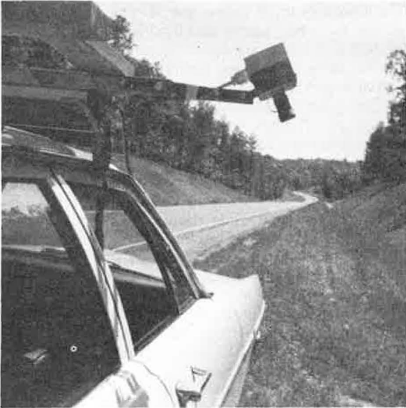
Figure 3. Side view of tracking system mounted on test vehicle.
