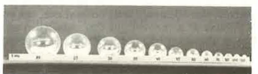
Figure 11. Embedment of 20-80 floating beads in a dry paint film 0.005 in. thick.
