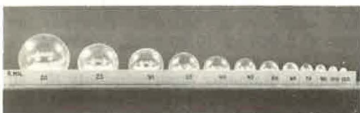
Figure 8. Embedment of 20-80 floating beads in a dry paint film 0.008 in. thick.
