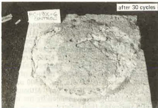
Figure 7. Surface of freeze-thaw specimens.
