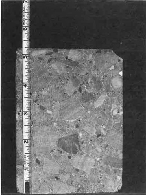
Figure 4. Cross section of core of polymer-impregnated bridge deck.
