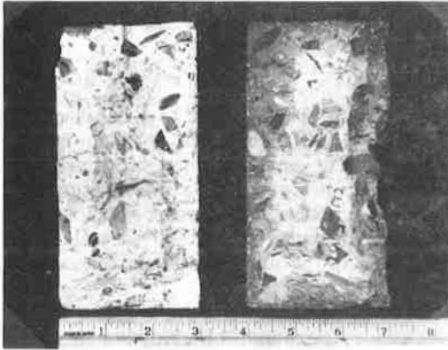
Figure 14. Acid-etched (left) and non-acid-etched (right) sections from specimen partially impregnated with sulfur.
