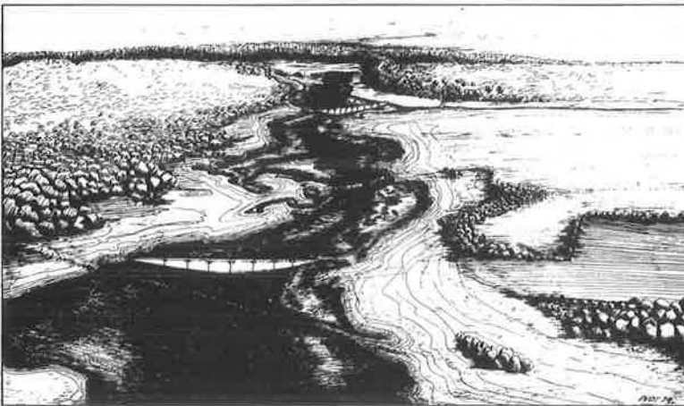
Figure 3. Silt barrier placement in Meginnis Arm.
